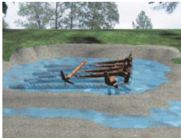
Step 6. Place a second cross spanning log.
