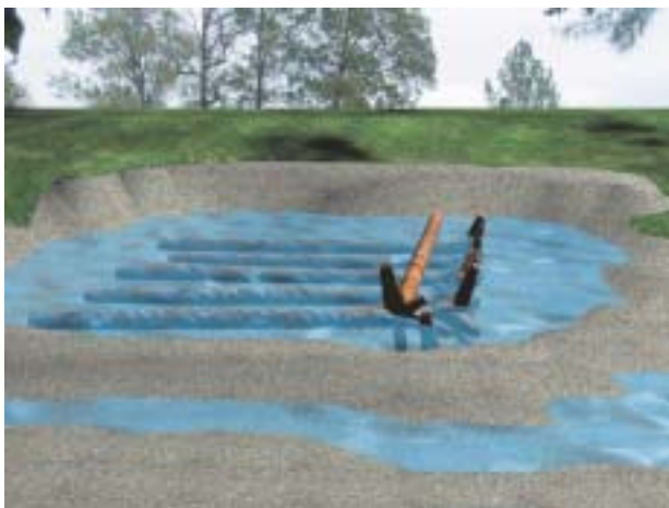
Step 4. Place first cross spanning log.
