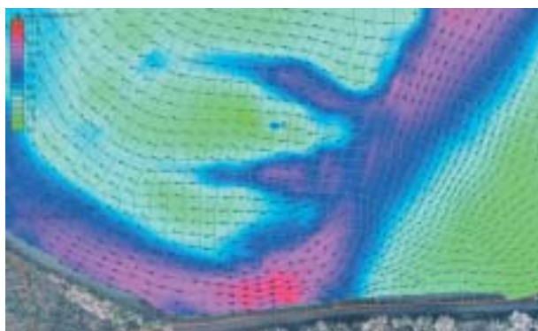
Figure 27 (below and right). Example output of 2D hydrodynamic modelling from the Hoh River ELJ project WA, USA. Courtesy T. Abbe. 27a (below) shows the situation before construction, 27b (right) illustrates the predicted changes after structure emplacement.
