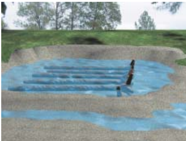
Step 3. Place key member logs parallel to the flow, root wads upstream.
