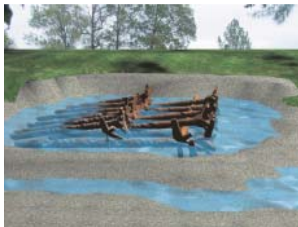
Step 7. Place a second row of longitudinal logs.
