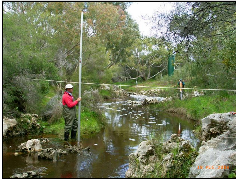
Plate 2. Example of undertaking channel cross-section surveys using dumpy, staff and tape measure (Hill River, August 2004).
