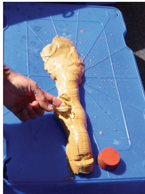
Figure 3: Sediment core taken from west of Parker Point, Dampier Port, showing the yellow clay-like material overlaying the original sediments
