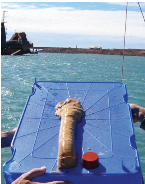
Figure 3: Sediment core taken from west of Parker Point, Dampier Port, showing the yellow clay-like material overlaying the original sediments
