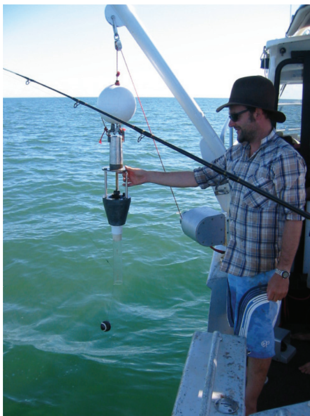
Figure 1. Wildco 2401-B20 KB heavy corer being deployed using the gantry and winch on the Department of Environment research vessel Zoila (note the spherical stopper attached to the fishing line and threaded through the core tube).
