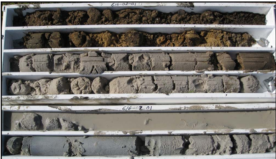
Figure 5: Photograph of a 6m soil core extracted from a site using sonic drilling.
