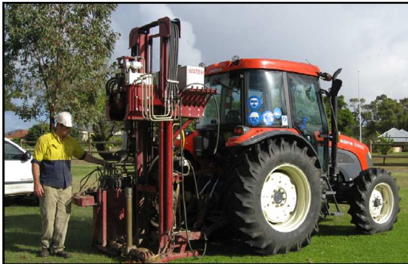
Figure 4: Photograph of the tractor-mounted sonic drill rig used for extracting soil cores.
