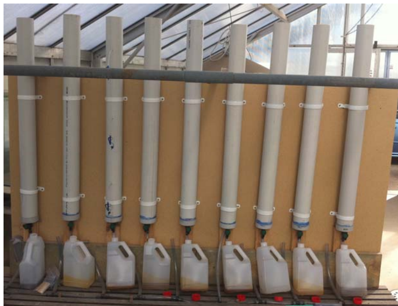
Figure 2. A photograph of the experimental set for oxidation and leaching of soil columns.
