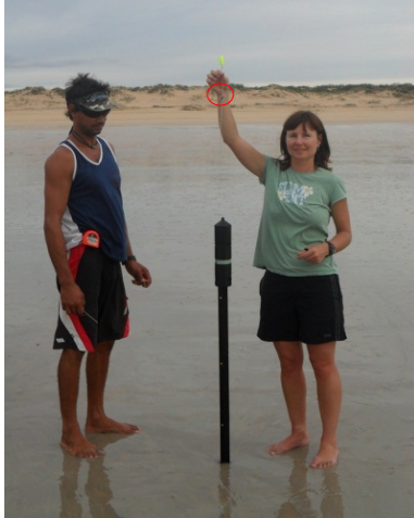
Figure 4. One of the receivers attached to a star picket. Michele holds up the synch tag (circled in red) with float attached with a piece of thick monofilament line.
