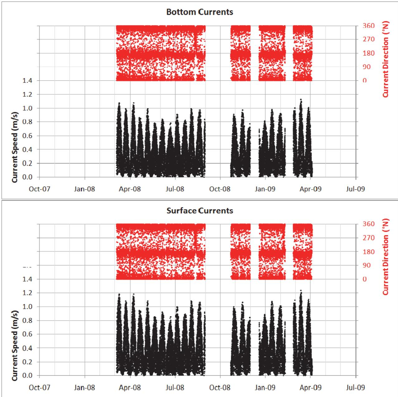
**Figure 3.4** Observed Currents at the offshore ADCP site
