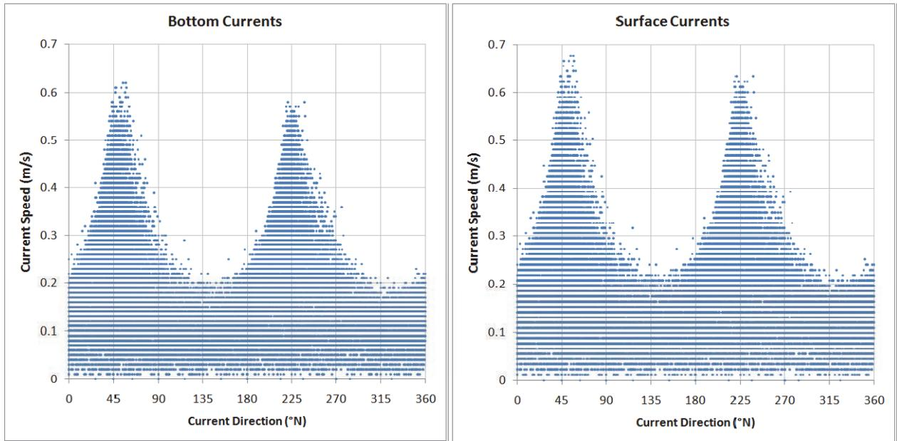
**Figure 3.7** Distributions of current speed and direction for the surface and bottom currents at the inshore ADCP site.
