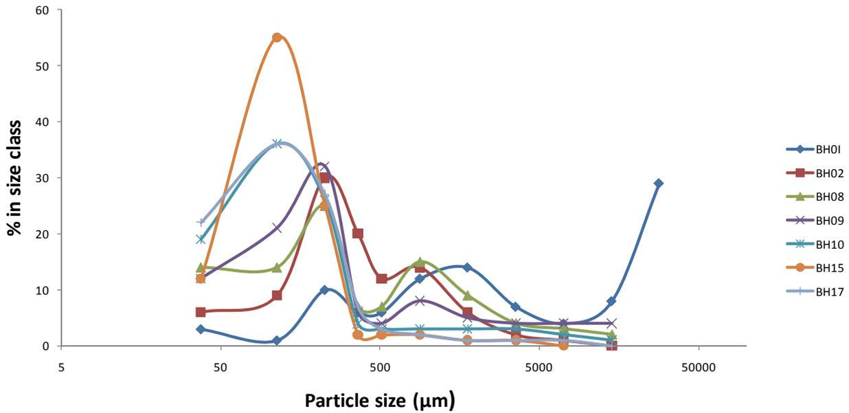
Figure 5.2 Grain size curves from AECOM borehole sediments
