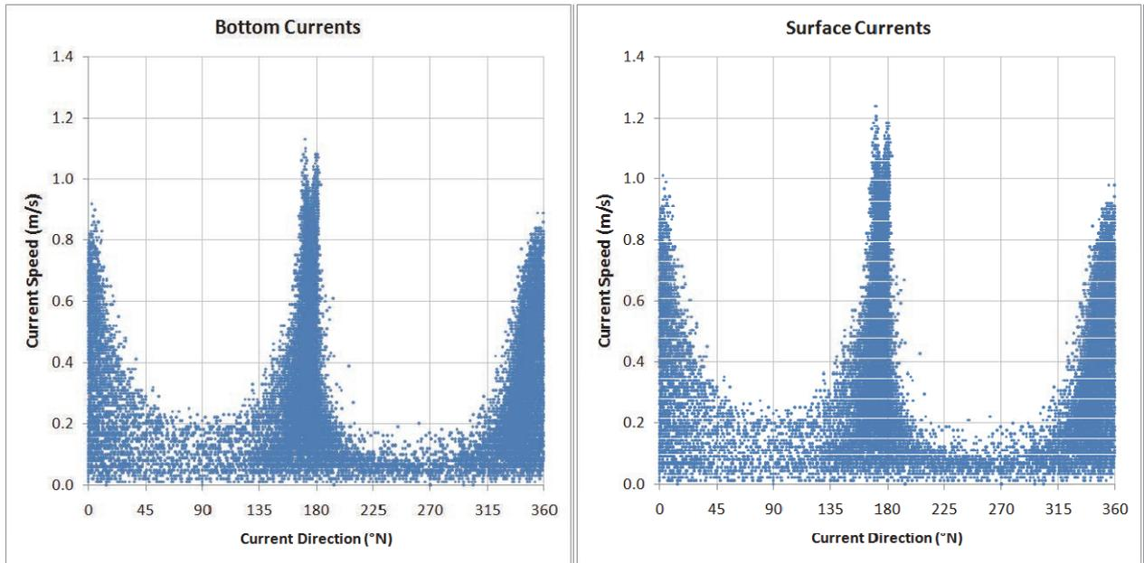
**Figure 3.5** Distributions of current speed and direction for the surface and bottom currents at the offshore ADCP site
