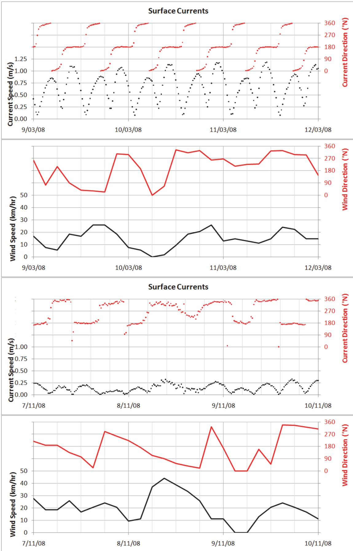
**Figure 3.8** Surface currents at the offshore site showing tidal characteristics without (upper) and with (lower) the influence of strong winds
