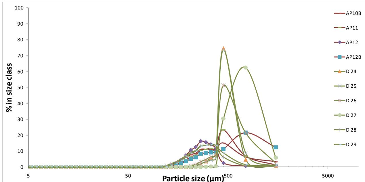
Figure 5.5 Grain size curves from Oceanica shoreline sediments
