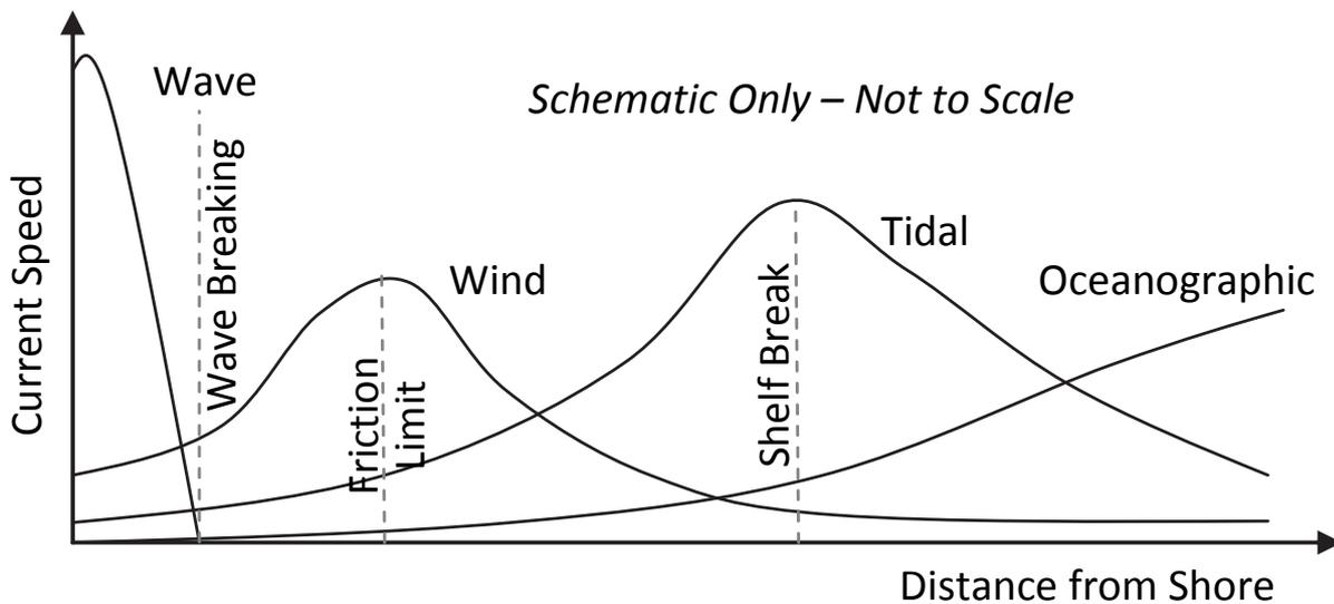
**Figure 3.2 Cross-shelf distribution of the principal driving mechanisms of currents**
