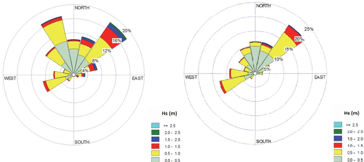
**Figure 3.10 Wave roses from ADCP deployments (left) offshore and (right) inshore**
