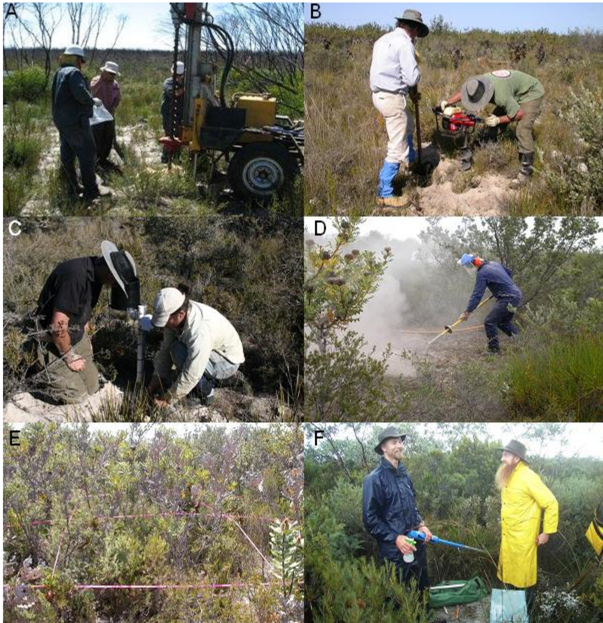
Figure 20. The monitoring program for the 'Last Stand at Bell Track' containment project included hydrological investigations (A); epidemiological studies of the pathogen (B); recording weather conditions on site (C), air spading to describe the root architecture of susceptible species (D), flora monitoring (E) and intensive sampling of the pathogen (F).
