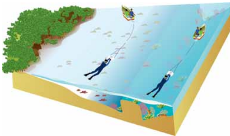
Figure 4. Manta tow survey technique.
