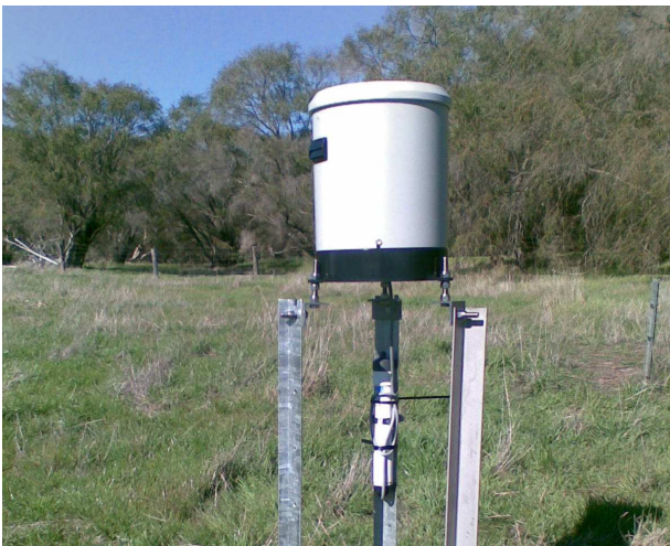
Photo 28: Tipping bucket rainfall recorders have been installed on 14 wetlands. Lake McLarty, Alan Clarke, 02Apr2012.
