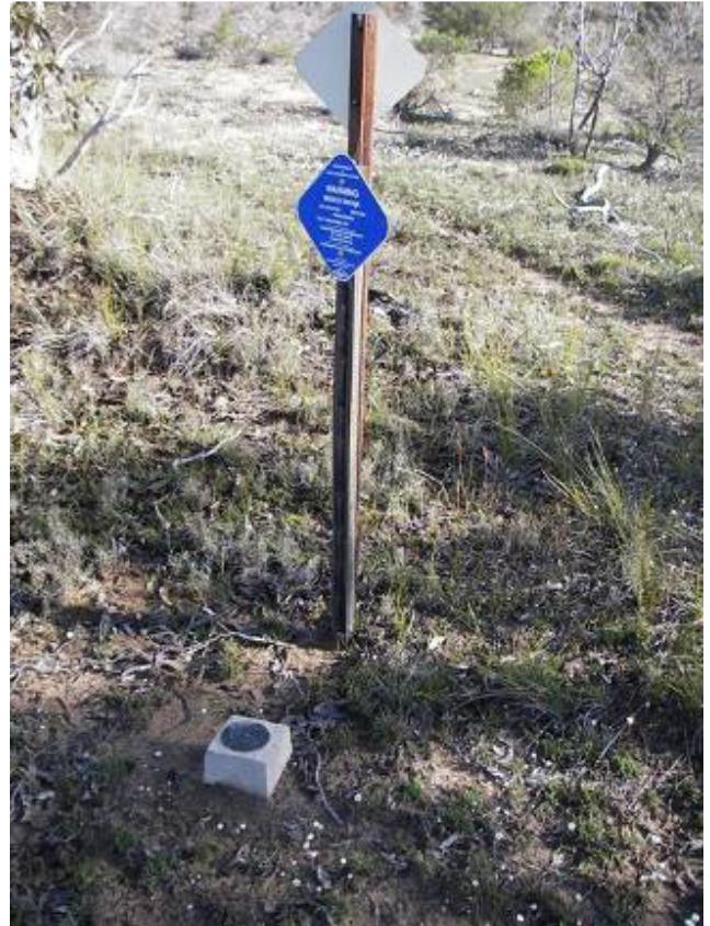
Photo 10: 'Landgate' Bench Mark and Witness Plate at 'Cranbrook 25812' in Nov 2008.
