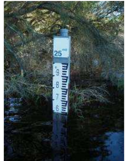
Photo 6: DoW water level gauge at Gibbs Road Swamp on 04Aug2008 read 24.59mAHD
