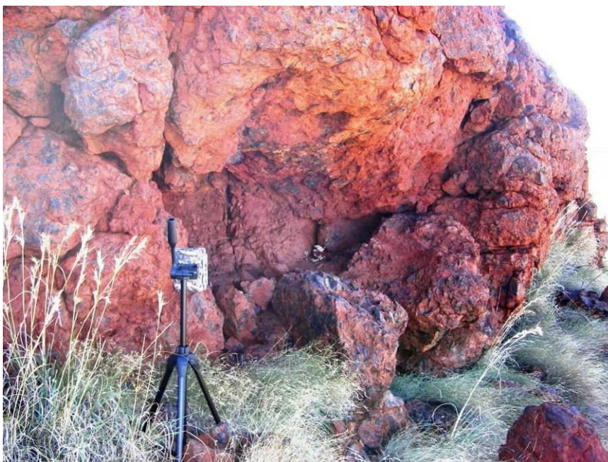
Figure 2. Example of a motion sensor camera set up on a tripod to detect northern quoll activity.
