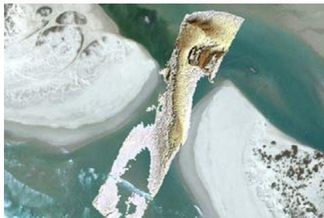
Figure 20. Overlay of a digital elevation model generated from the lidar data measured at the Murray mouth and aerial photography.
