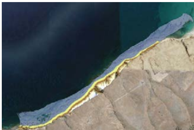
Figure 19. Overlay of a digital elevation model generated from the lidar data measured at Sellicks Beach and aerial photography.
