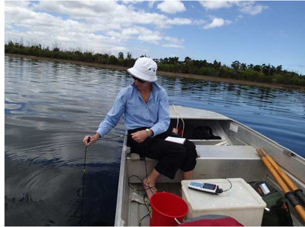
Photo 8: Y. Winchcombe lowering the conductivity / salinity / temperature probe at Lake Jasper on 04Nov2015.
