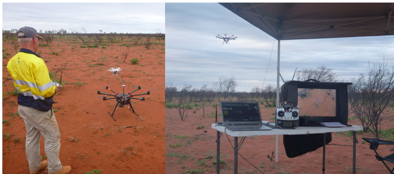
Figure 9. The two rotary wing RPA and live HD video feed that was trialled in 2015.
