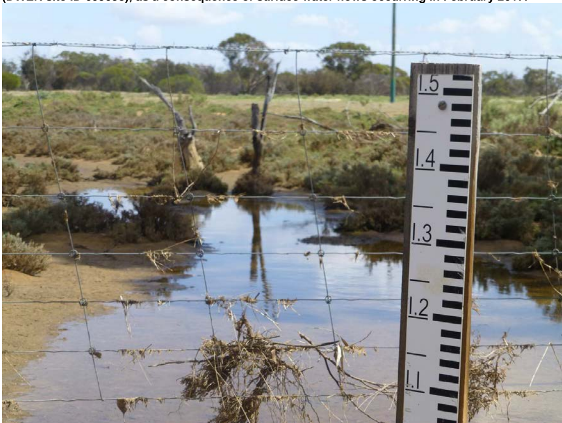
Figure 3. Westwards photograph of site 01DEC01, located at outlet of the western tributary of Management Area MA1. Note the trash evident on the fence line, estimated to be at 1.45 m on the staff gauge (photograph Darren Farmer).
