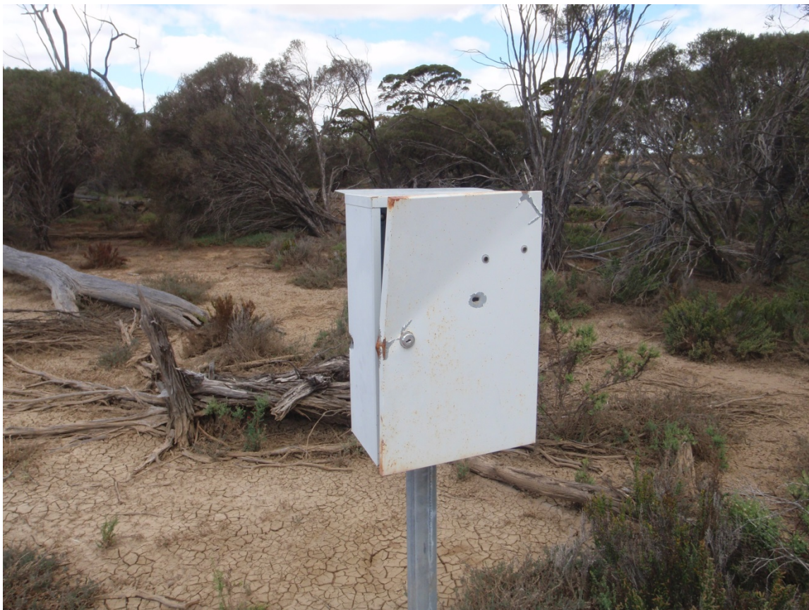
Figure 5. Data logger cabinet at site 03DUL06 located in the waterway east of Oval road. Note the small-calibre gunshot entry points on the door and evidence of forced entry.
