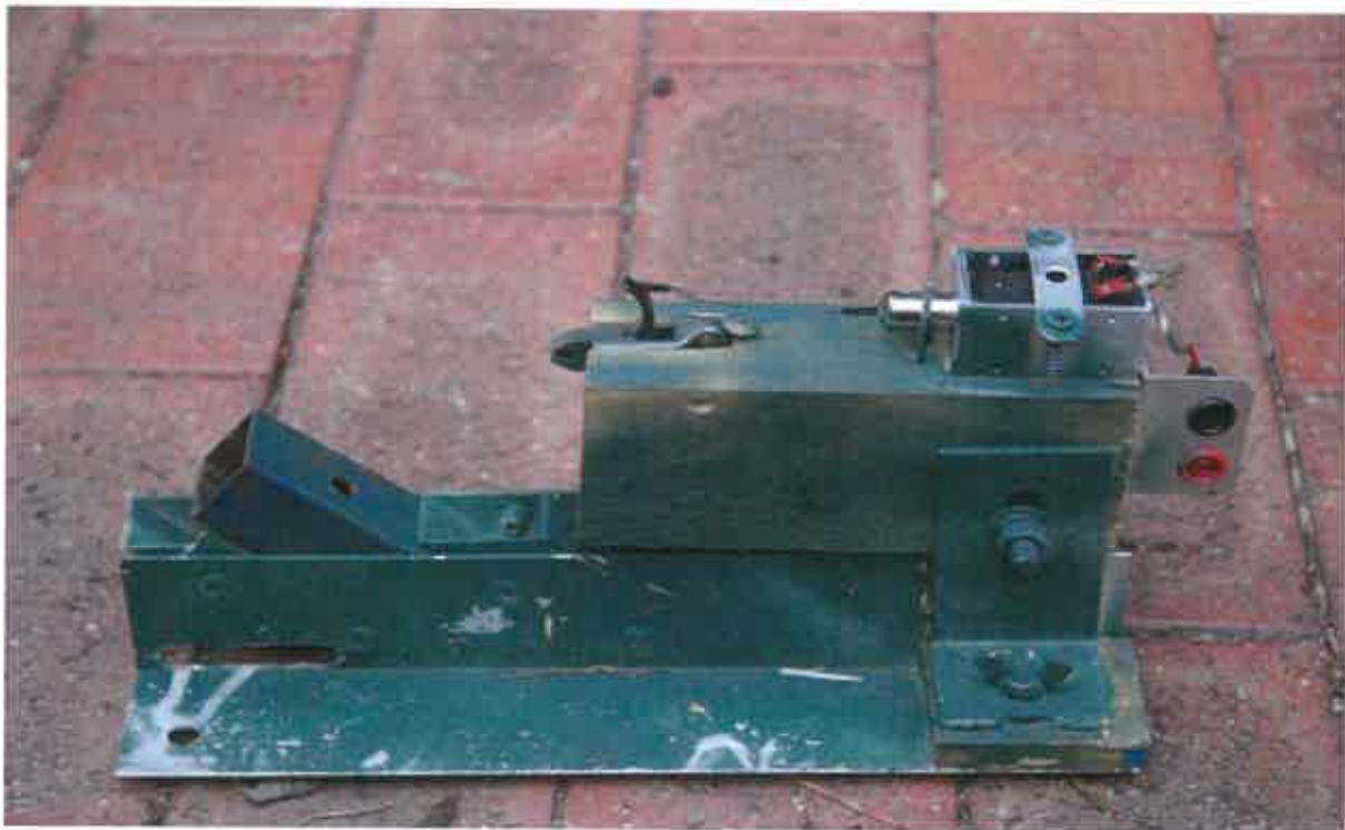
Figure 4 The release mechanism showing from left to right, the guide pole base set at a predetermined angle, the bow-string release, the solenoid and the electrical plug ports.
