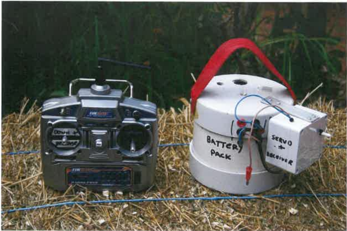
Figure 5 The transmitter (left), and the receiver/battery pack (right). The battery pack, servo and receiver have been combined into one unit for convenience.
