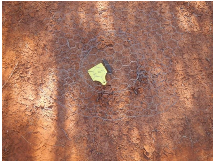
Plate 4: A caged bait on clayey soil – bait longevity trial.
