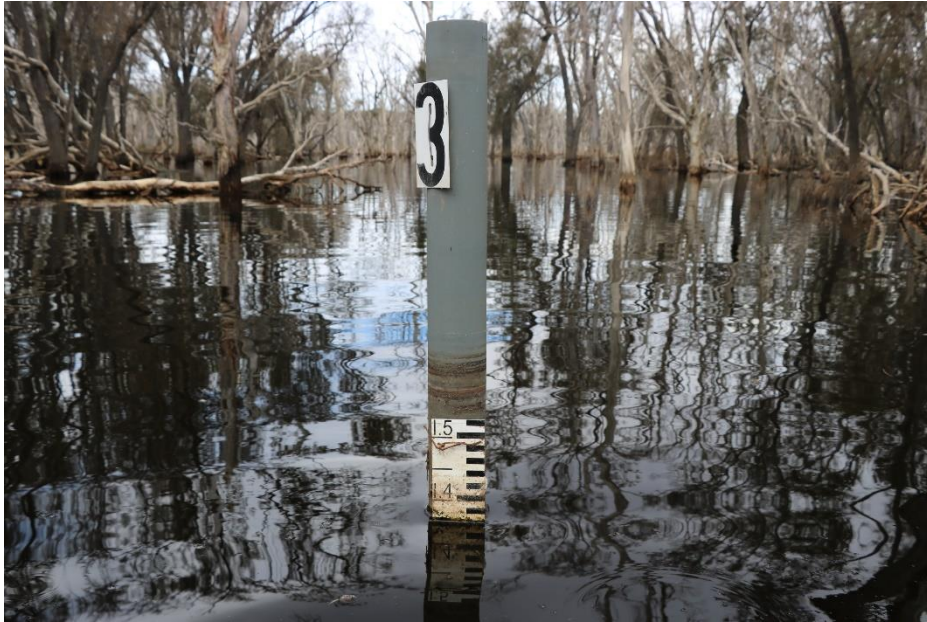
A gauge board. The alternating black and white bars are 1 cm wide with the measure commencing at the bottom of each bar. The water level at this gauge board is 1.37 m.
