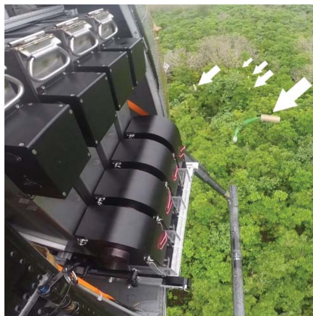
Fig. 6 Bait cartridges dispensed in flight.
