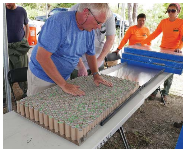
Fig. 3 Bait cartridges are inspected for manufacturing imperfections or shipping damage that might impede smooth feeding and ejection.
