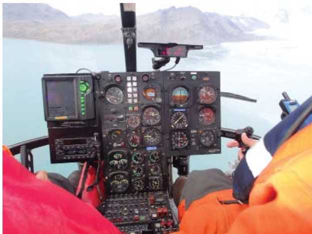
Fig. 4 TracMap™ GPS guidance equipment fitted to South Georgia Heritage Trust aircraft, 2015.
