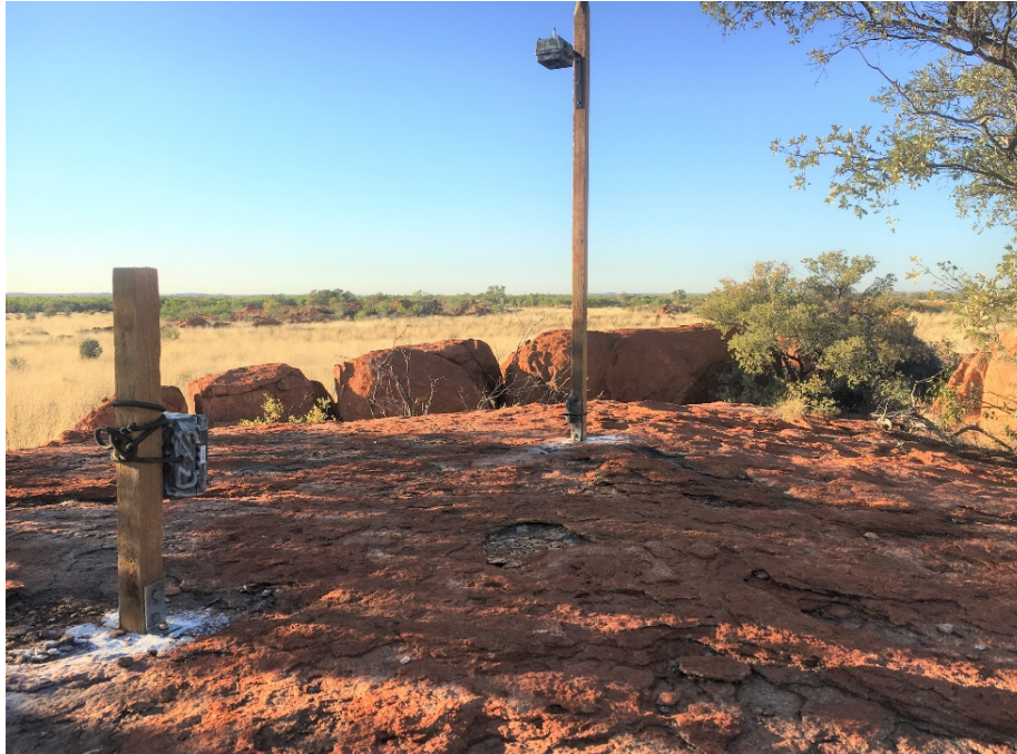
Figure 4. A comparison of vertical and horizontally oriented camera traps, with a bait pod secured to the stake with the downward-facing camera. Vertical orientation reduces the rate of 'false triggers' by reducing vegetation in the frame. Although this strategy reduces the field of view from several hundred m 2 to approximately 2.55m 2 , detectability for small species such as northern quolls appears to remain comparable and permits individual identification via spot pattern.
