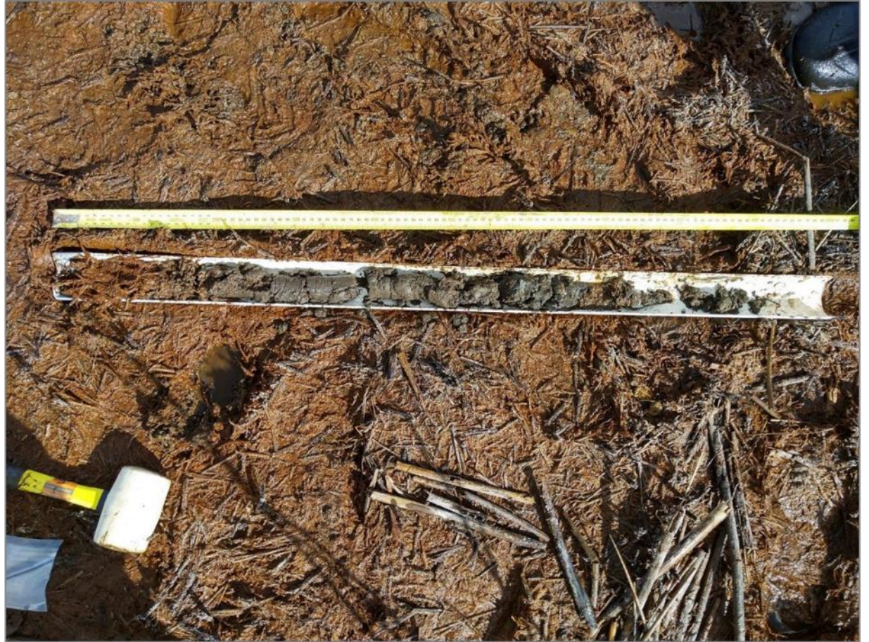
Transect 2 site TGN10b – soil water sampling and peat core (fibric peat stained by iron oxyhydroxide - sulphide minerals grading to competent peat (higher carbon and clay material content); left to right)
