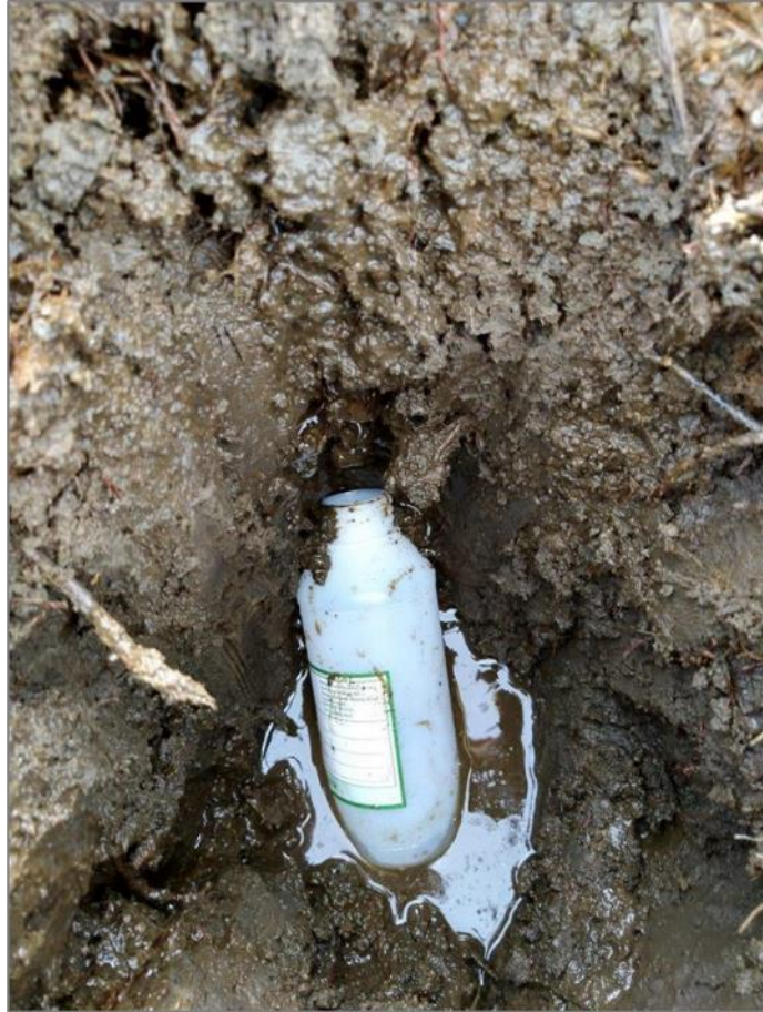
Transect 2 site TGN10b – soil water sampling and peat core (fibric peat stained by iron oxyhydroxide - sulphide minerals grading to competent peat (higher carbon and clay material content); left to right)
