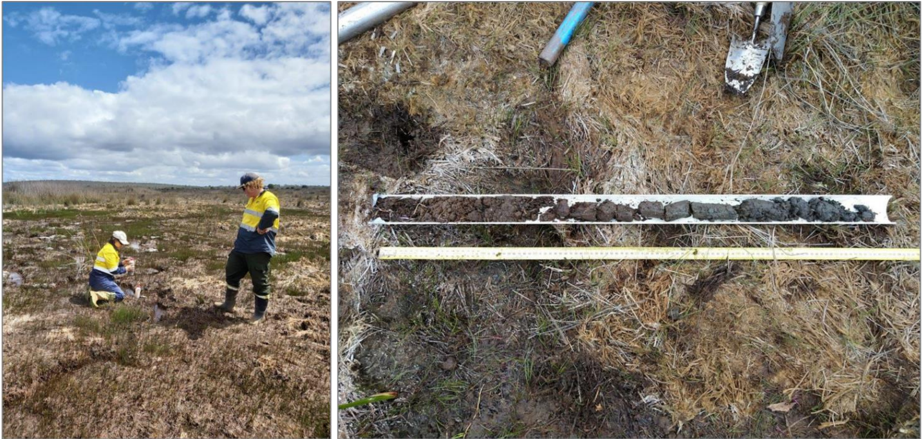
Transect 2 site TGN9b – water sampling and peat core (fibric peat grading to competent peat (higher carbon and clay material content); left to right)
