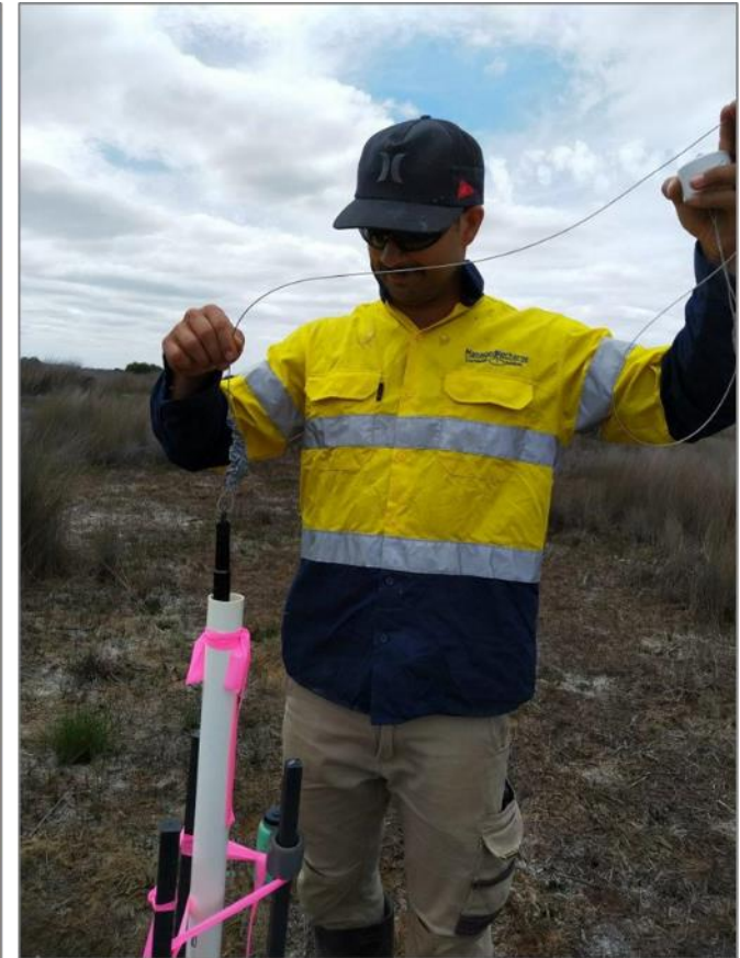
Transect 2 site TGN10b – mini piezometer construction, showing stick-up and data logger installation to measure hourly groundwater level, temperature and electrical conductivity
