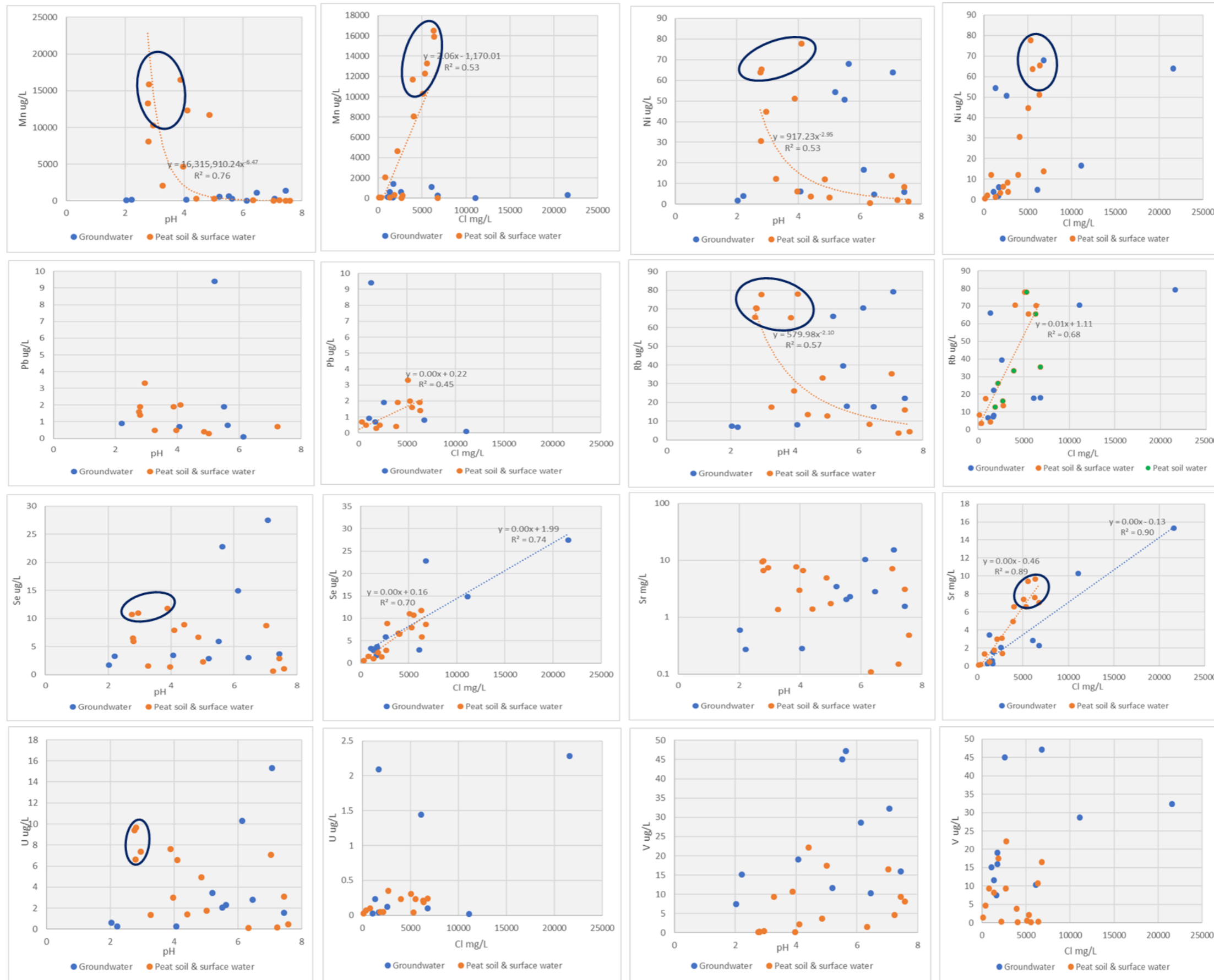
Bivariate plots; concentration (pH units, mg/L or µg/L) minor ions (metals & metalloids) with respect to pH and chloride; surface water data from five lakes and groundwater & peat soil water from four lakes within the Muir-Byenup Ramsar site (2015 to 2019) (NB trendlines & correlation coefficients are present where relationships were observed; 2019 data generally have higher concentrations (see Appendix 3) and are circled in black where they were measured & verify trends or form a population
