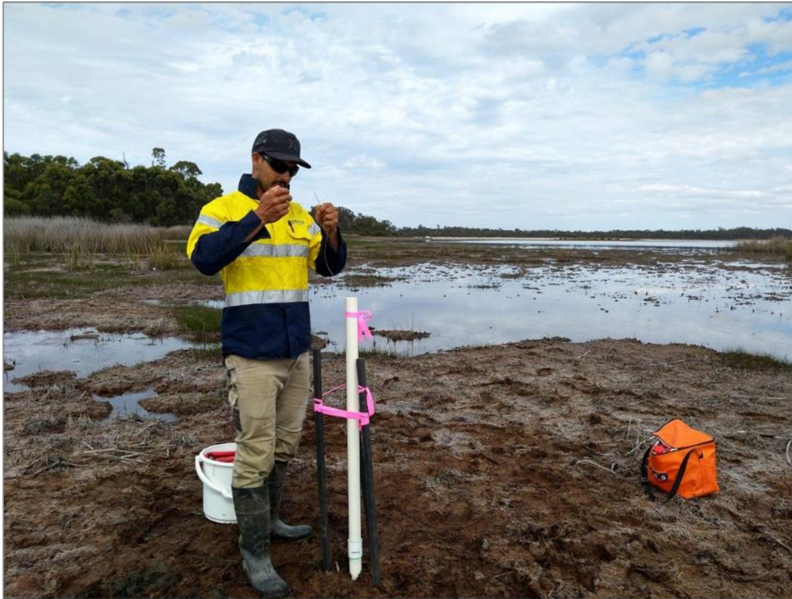
Transect 2 site TGN10b – mini piezometer construction, showing stick-up and data logger installation to measure hourly groundwater level, temperature and electrical conductivity
