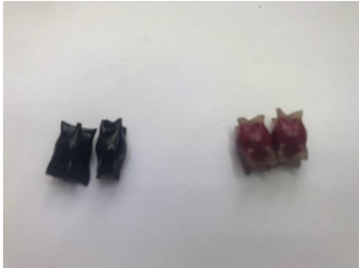
Plate 8. Apo-HSDVs, 'blackening' of the coating matrix on the left, clear HSDV (containing Rh B) on right.
