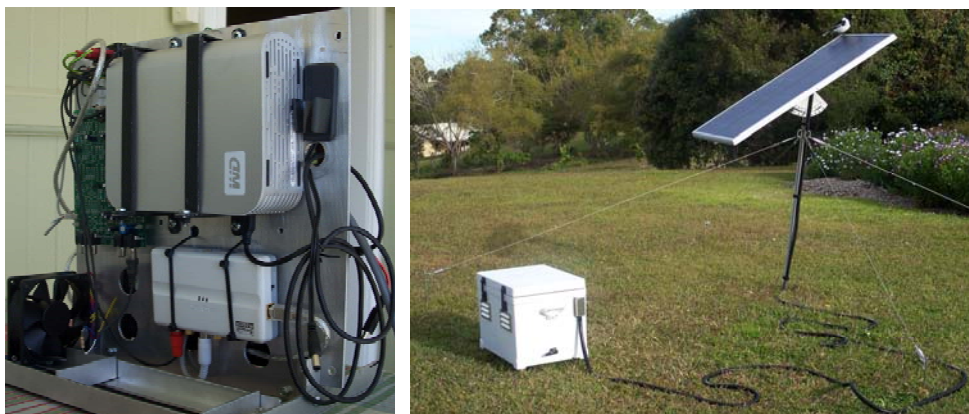
Figure 1. The recorder with a terabyte HDD and the recorder in the field
