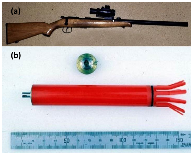
Figure 3 PAXARMS biopsy system (a) Assembled 0.22 calibre rifle with Pro-Point red-dot sight. (b) Biopsy dart and biopsy tip. Photos taken from Murdoch University Cetacean Research Unit.
