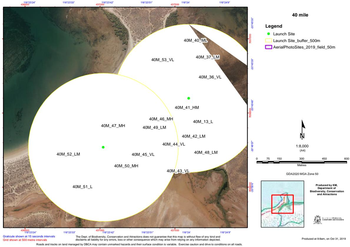
**Figure 4:** Field trip map for planning site capture with suggested locations for launching the RPA and the flying distance limits (within a 500m line of sight buffer). With multiple RPA operators this can help plan who will fly each site when in the field.
