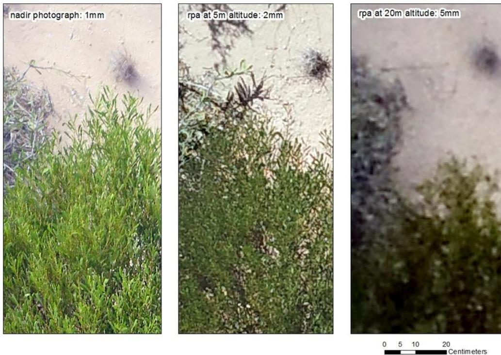
Figure 3: A comparison of imagery from nadir photography (1 mm resolution), RPA at 5 m altitude (2 mm) and RPA at 20 m altitude (5 mm).
