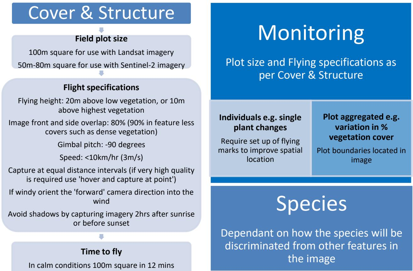
Figure 1: Flowchart of field plot size flying specifications for obtaining different ground measures.
