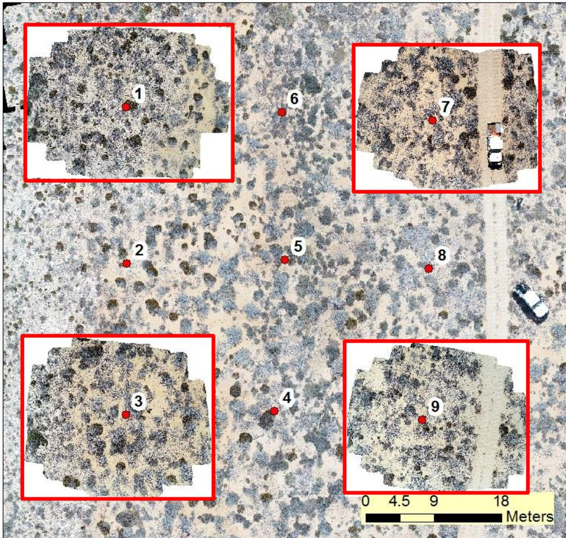
Figure 8: Configuration of RPA image captures at monitoring sites on DHI (red boxes).
