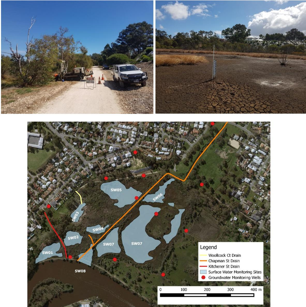
Figure 3: Installation of groundwater monitoring wells MW04D (top left); MW04S (top right) and locations of drains, groundwater monitoring wells and surface water monitoring sites.
