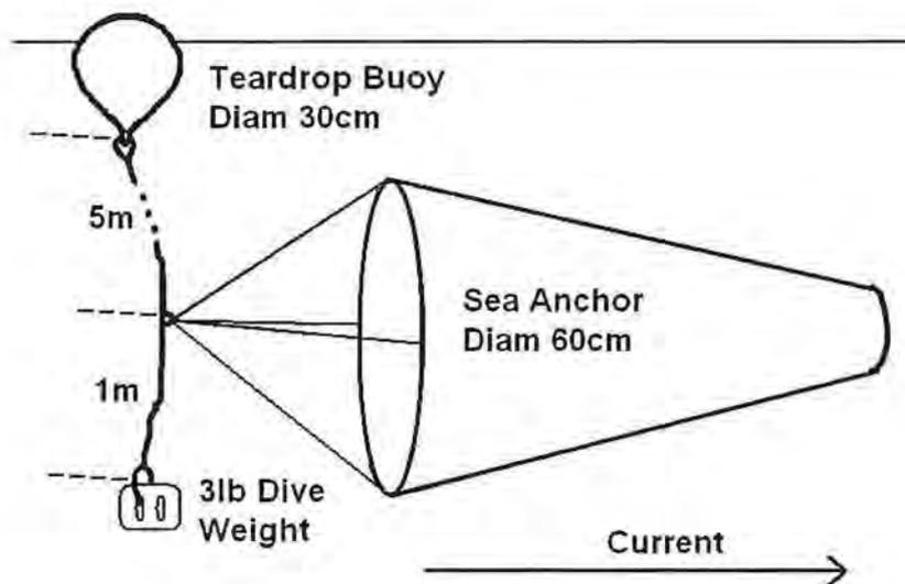
Figure 4.2: Configuration of drogue used to determine current speed and direction.
