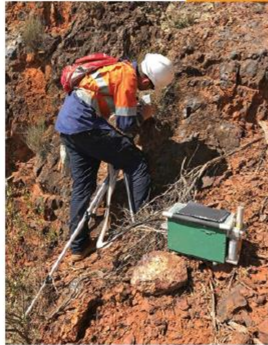
Ecophysiological assessments of Tetratheca erubescens using a gas exchange analyser to determine photosynthetic rates and fluorescence. Photo: Wolfgang Lewandrowski
