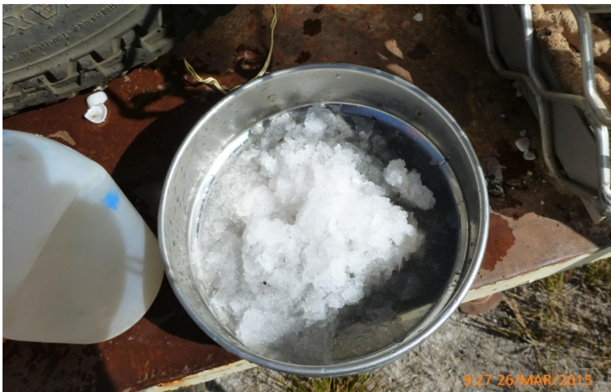
Figure 5: Suspended salts taken out of solution during field sampling (Lizamore 2015)
