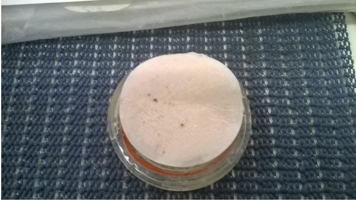
Figure 6: Salt crystallisation on paper filters during filtering (Lizamore 2015)
