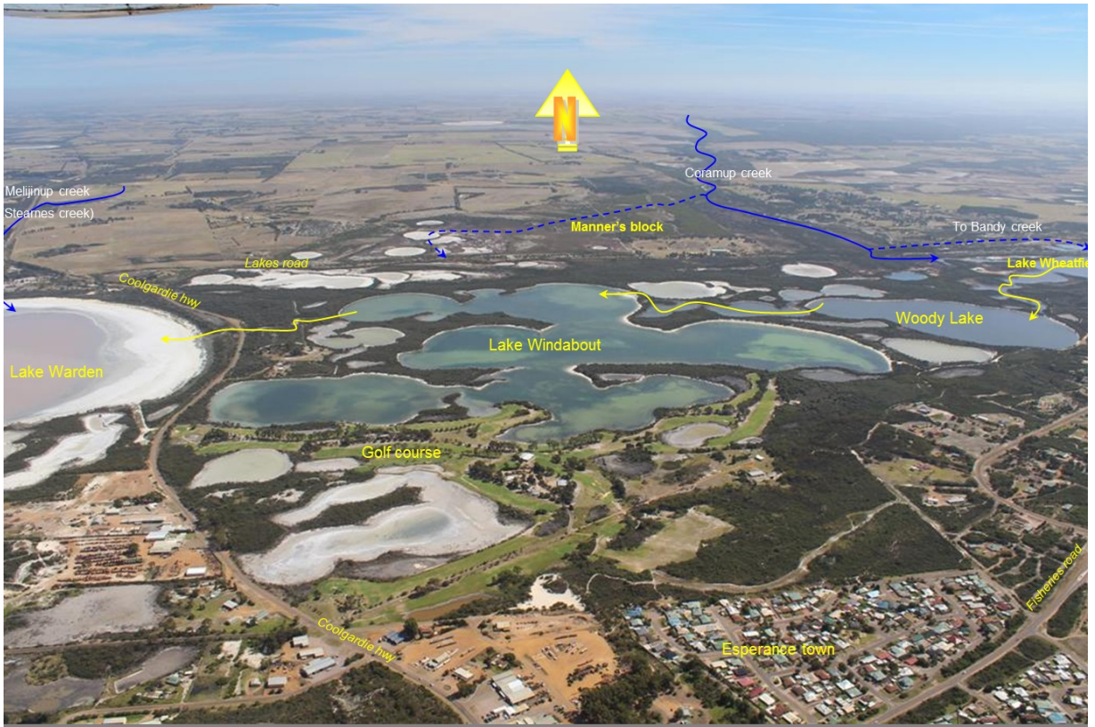
Figure 10. Flow paths of the Central Suite, as seen looking north.
