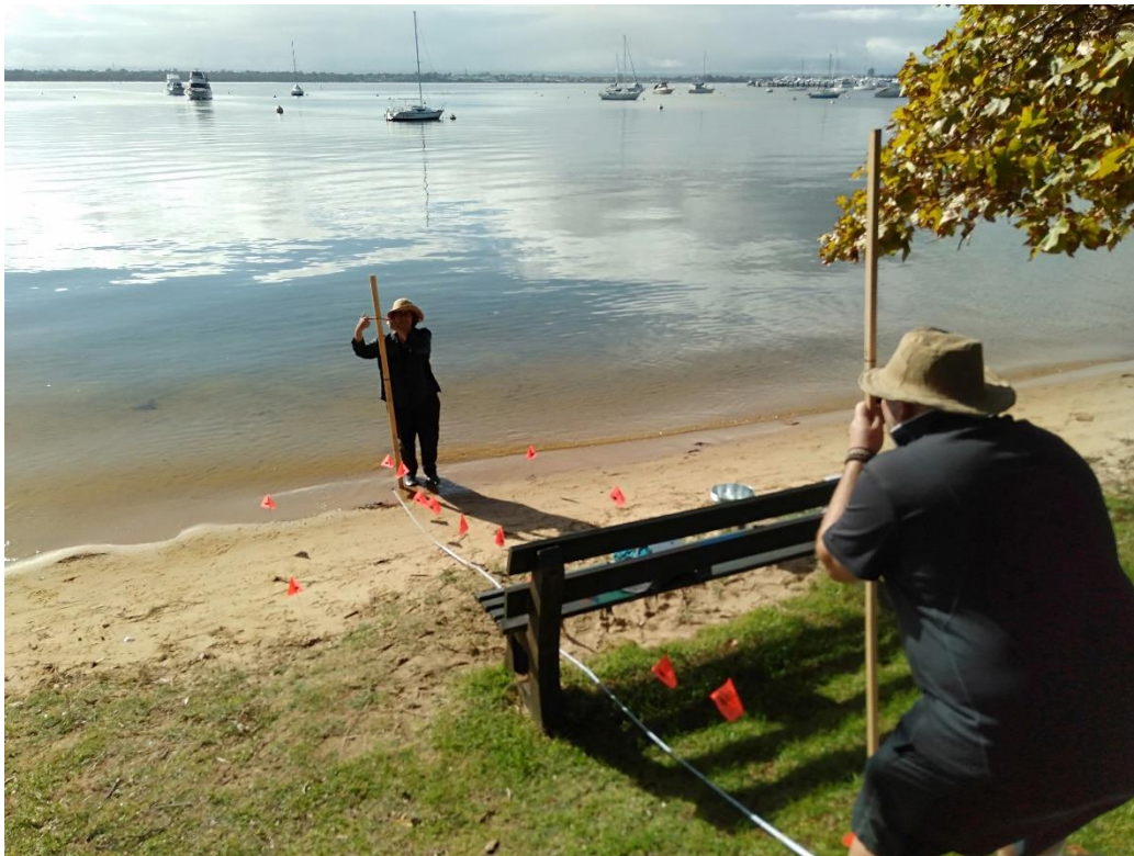
Figure A1.6. Taking bank height and slope measurements.
