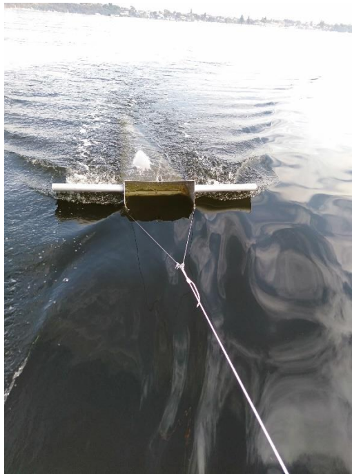
Figure 2 A deployed manta tow net collecting plastic samples
