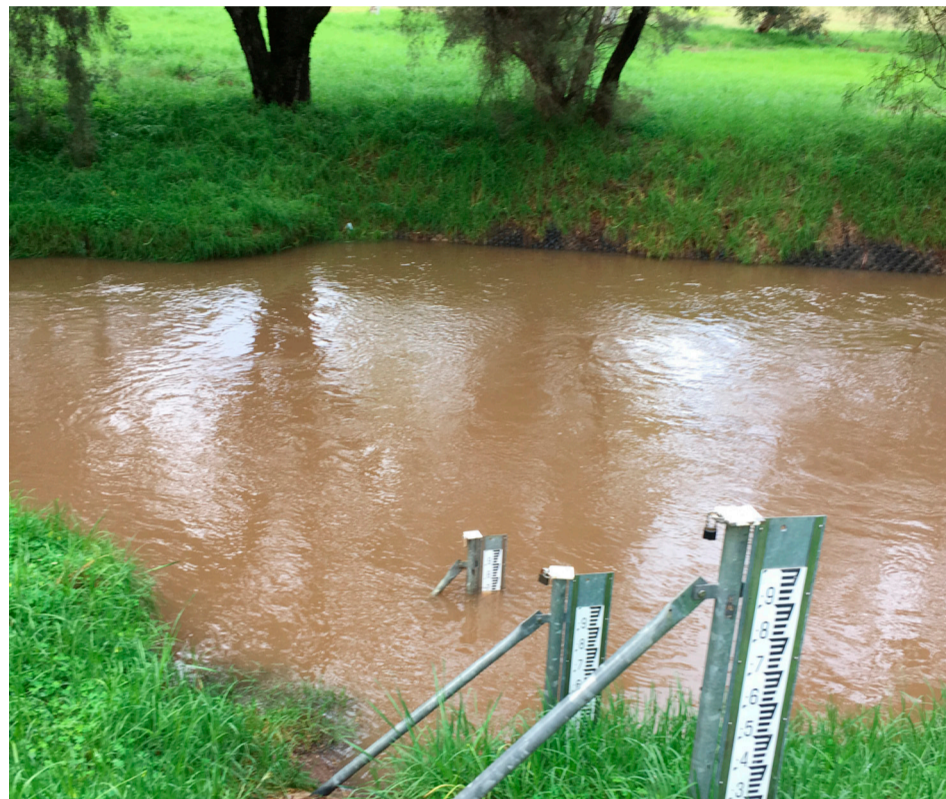
Staff gauges at the Upper Canning sampling site following heavy rainfall, August 2017. Photo: Dominic Heald
