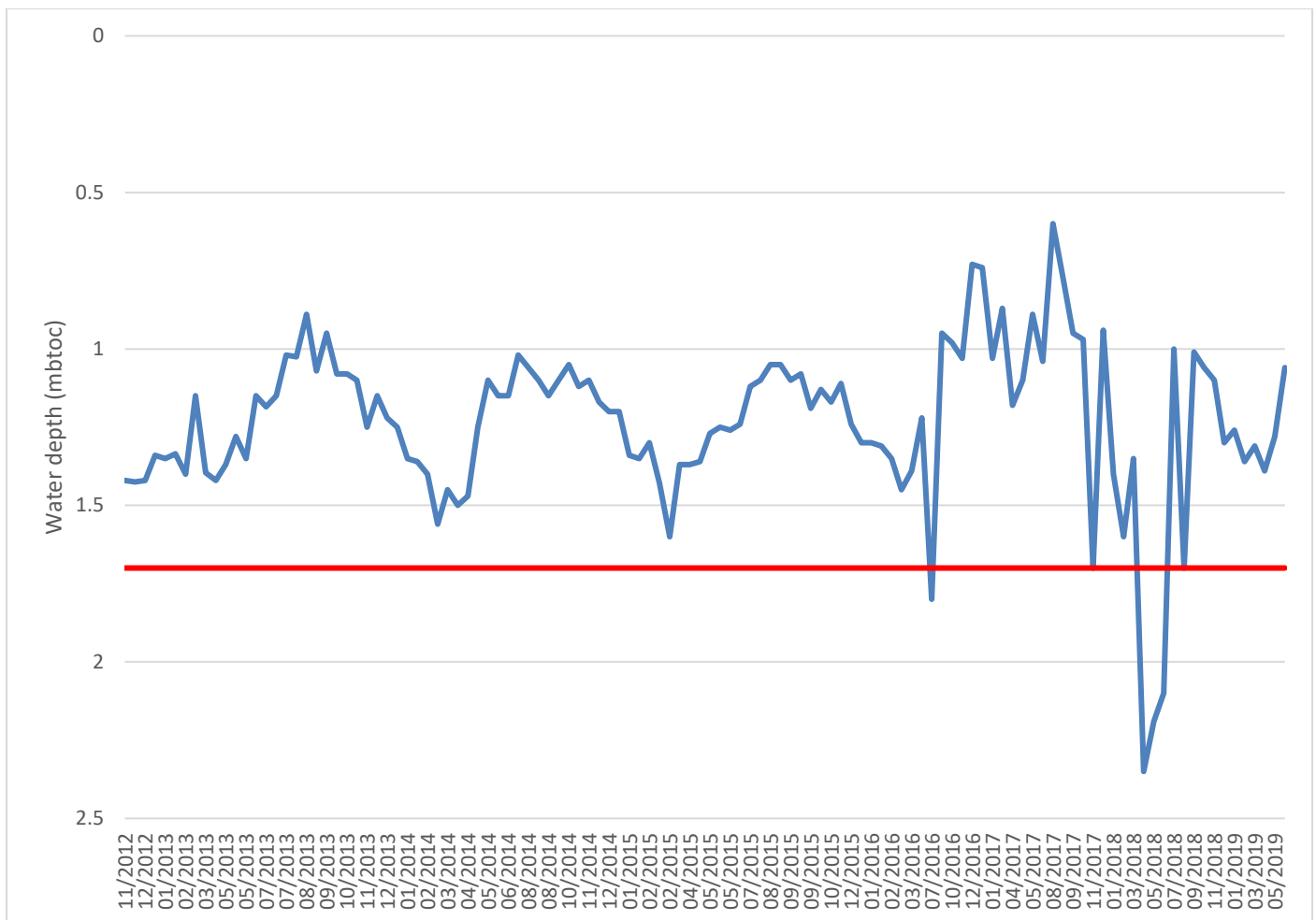
Figure 4. Water level (blue line) and trigger depth (red line) from Karara monitoring bore (located -29.452309; 115.5069797), from 2012 to 2019.
