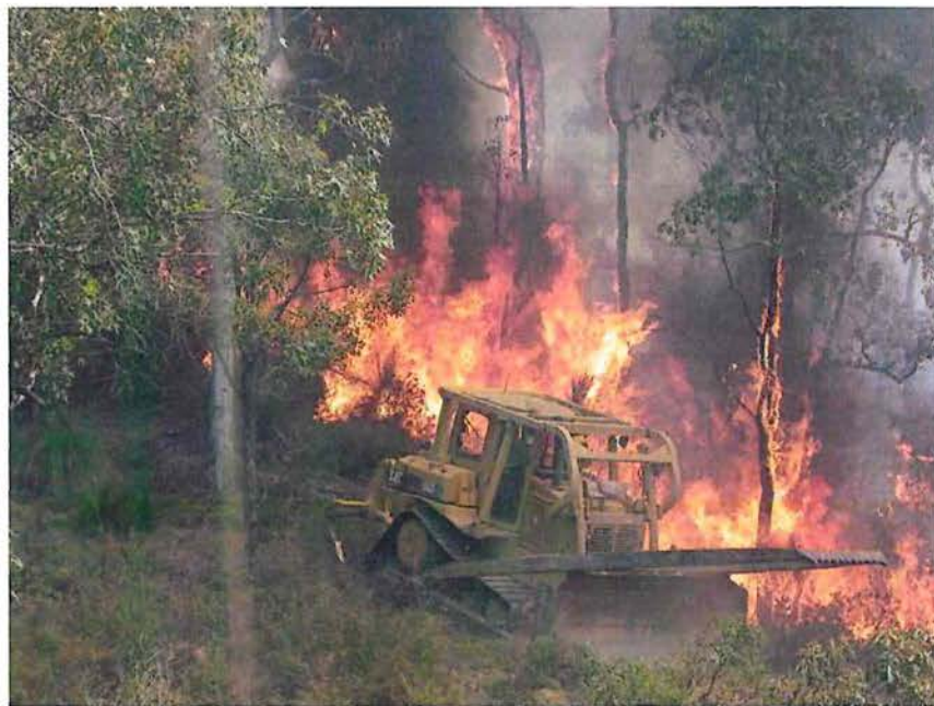
A bulldozer simultaneously knocking down a fire and constructing a containment line. A fire tanker is nearby in support but out of photo shot.
