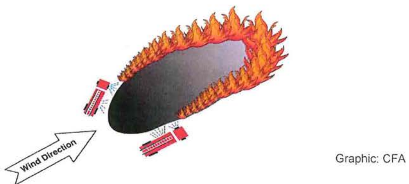
Flank attack on a fire. Tankers have commenced attack from the tail fire
