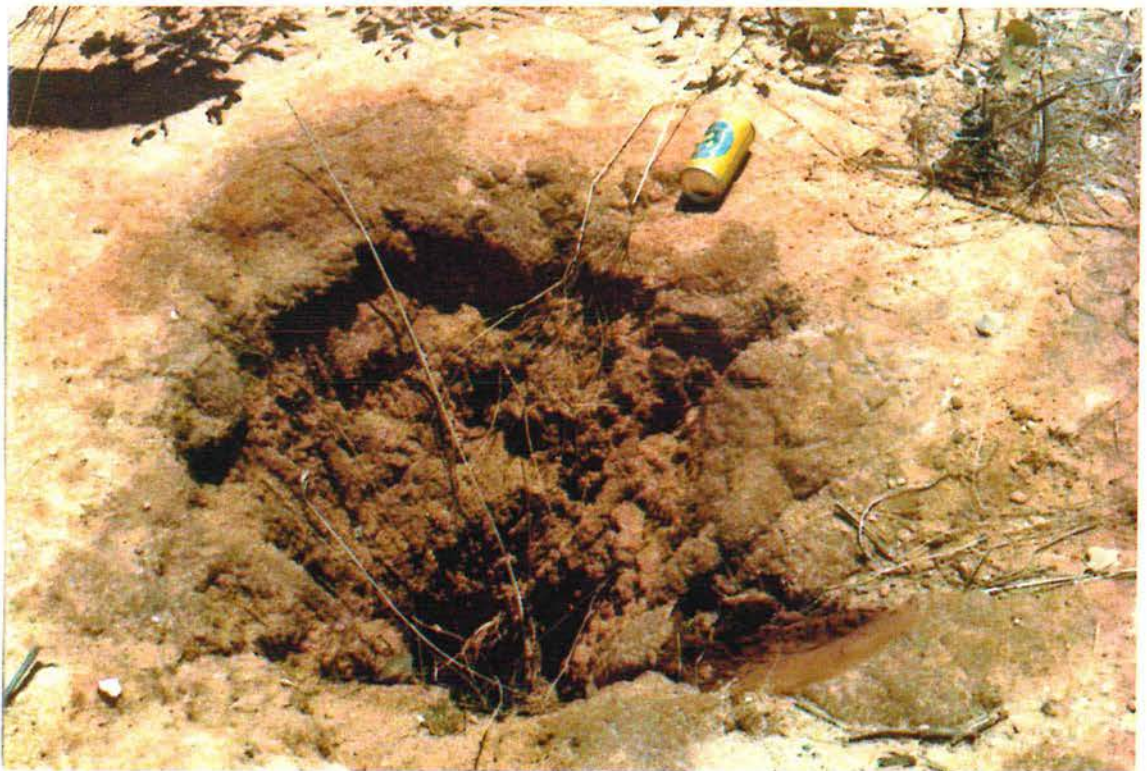
Fig. 6 An example of poor practice where no shothole cap was used and tamped back to surface.
