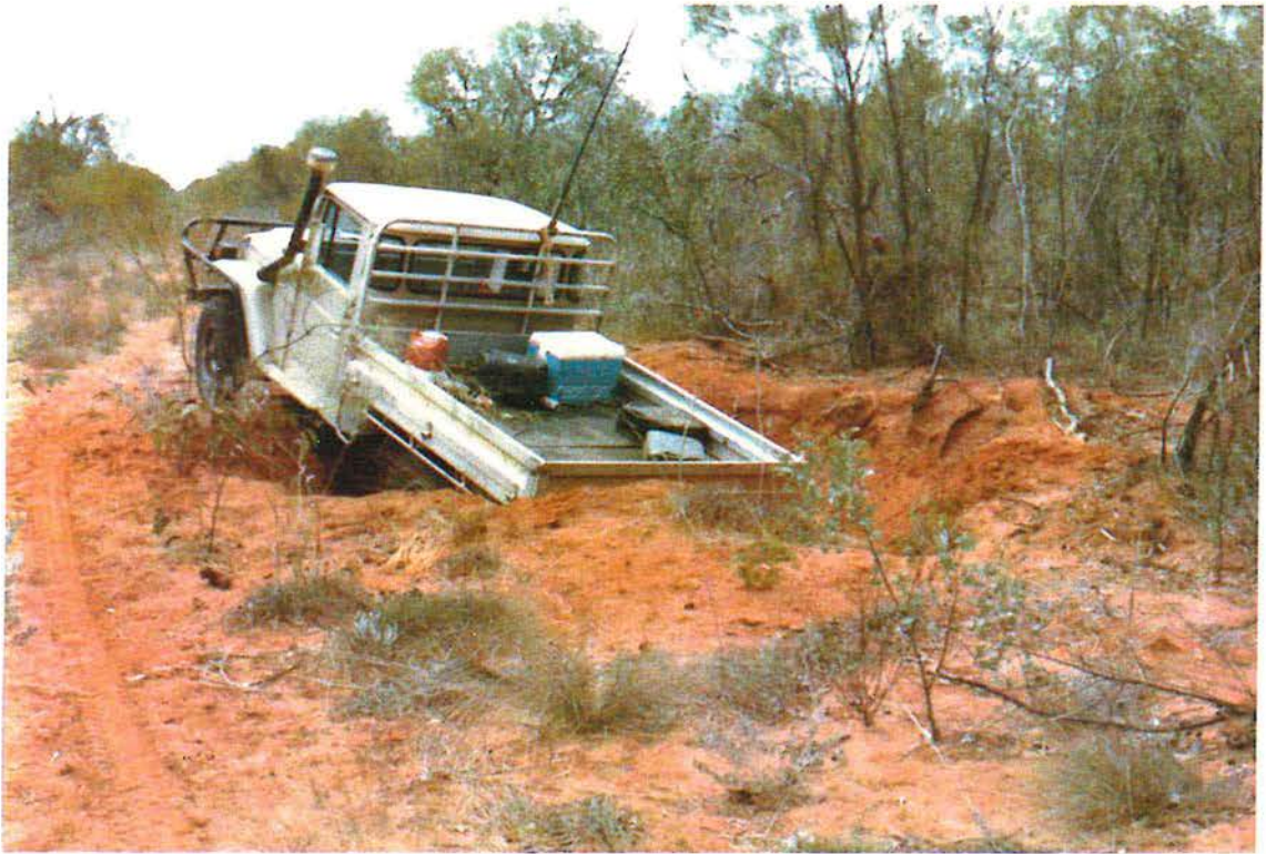
Fig. 5 Falling into a shothole drilled on-line, see fig. 6.
