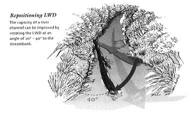
Figure 8: Repositioning large woody debris (Gippel et al., 1998).
