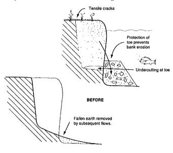
Figure 6: The use of structural works, such as a rock toe, will prevent the process of undercutting (adapted from Raine & Gardiner, 1995).
