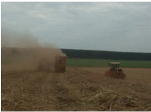
Figure 4.1 Trash recovery for cogeneration in Brazil by baling the trash after machine harvesting.
