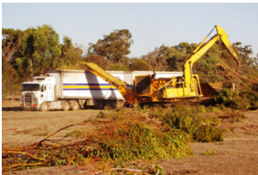
Figure 2.9 Loading a chip truck with mallee biomass using a roadside chipper
