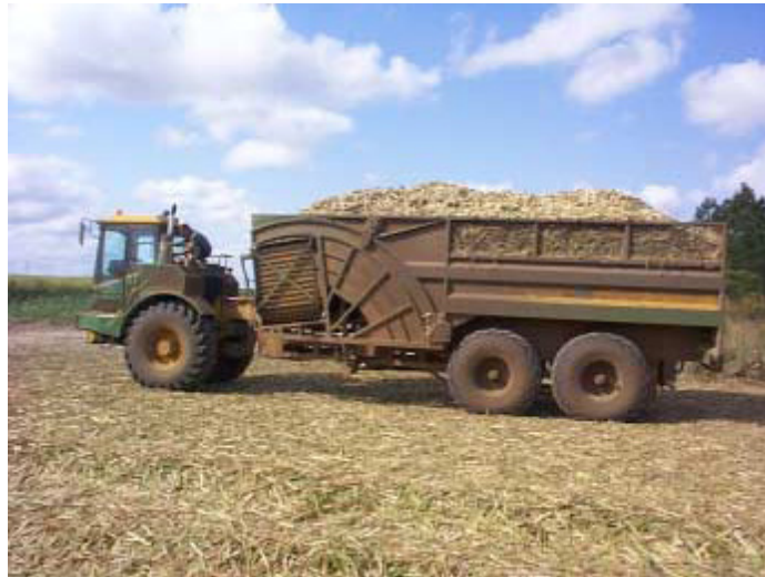
Figure 3.3 Articulated self-propelled with end lift and cross elevator unload
