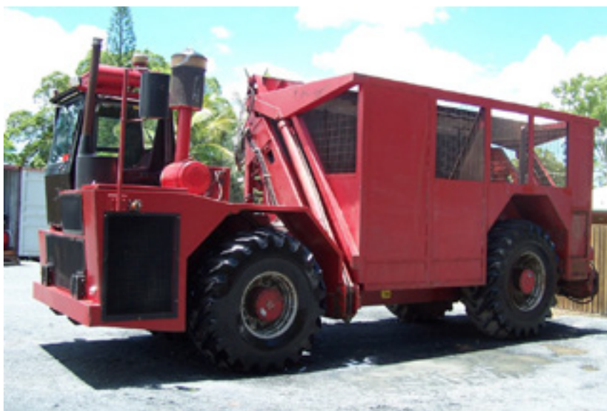
Figure 3.5 Self-propelled with side tipper (power haul)
