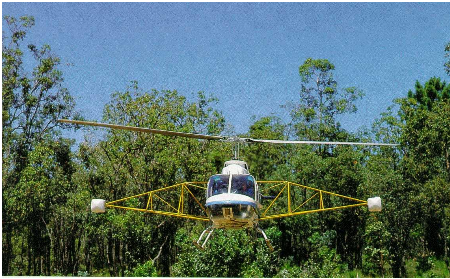
Figure 3: A Bell 206B Jetranger helicopter with boom mounted camera pods used in the jarrah inventory.
