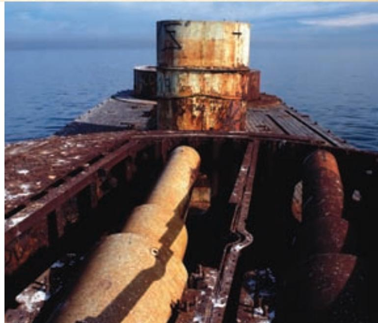
Her main armament consisted of four 10-inch muzzle loading guns mounted in two turrets. *Cerberus*' guns were capable of firing a round every 1.5 minutes; exceptionally fast for the standards of the day. She also had ballast tanks that could be filled to sink the hull and lower her freeboard to further reduce her profile in battle.
