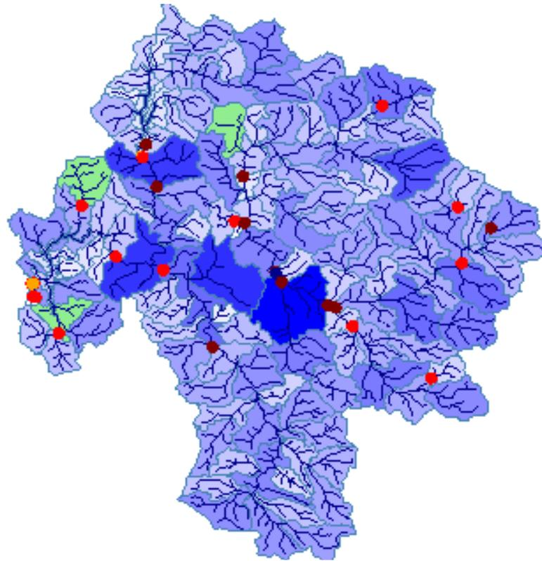
**Apx Figure B.3 Example of hydrological response units (HRUs) from LUCICAT. The runoff for each HRU, illustrated by the colours, is routed to the catchment outlet using a Muskingham method. The reporting nodes, catchment outlet and dams are indicated by dots of different colours**
