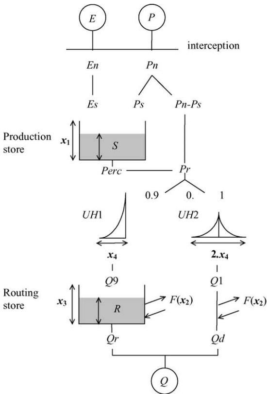
Apx Figure B.1 Schematic of the GR4J model (Perrin, 2003)
