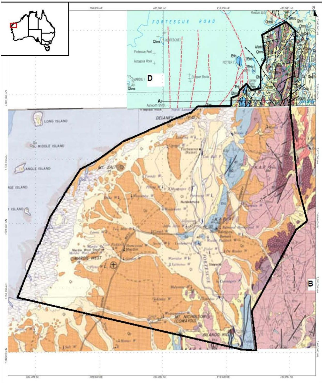
Figure 4.6 Surface geology of the Lower Fortescue River catchment and groundwater model boundary (MWH, 2010a)
