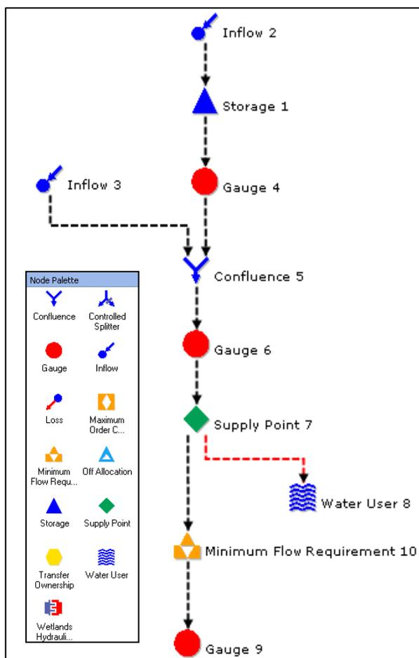
Figure 3.2 A schematic of a simple river network prepared in Source for river system modelling
