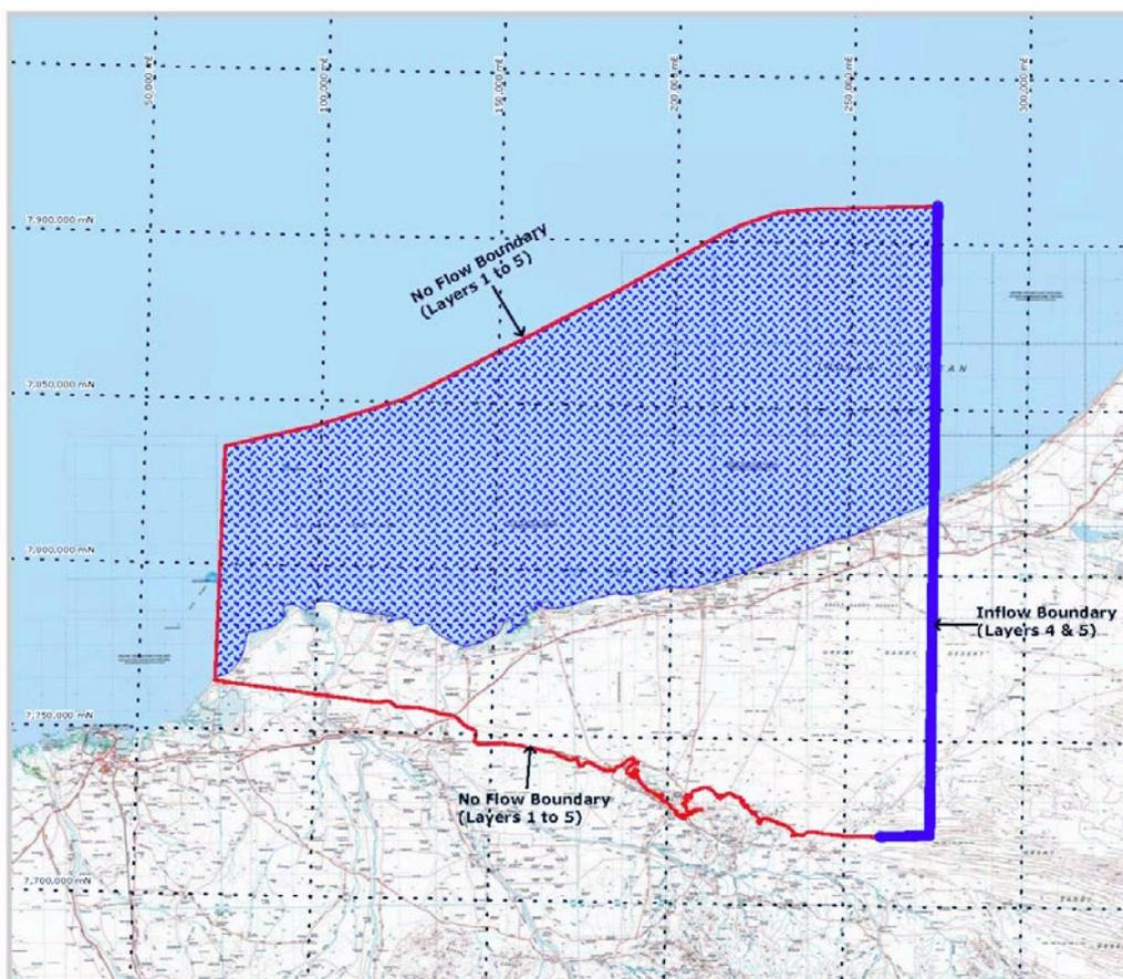
Figure 4.3 A map showing West Canning Basin groundwater model extent and boundary conditions Aquaterra, 2010)
