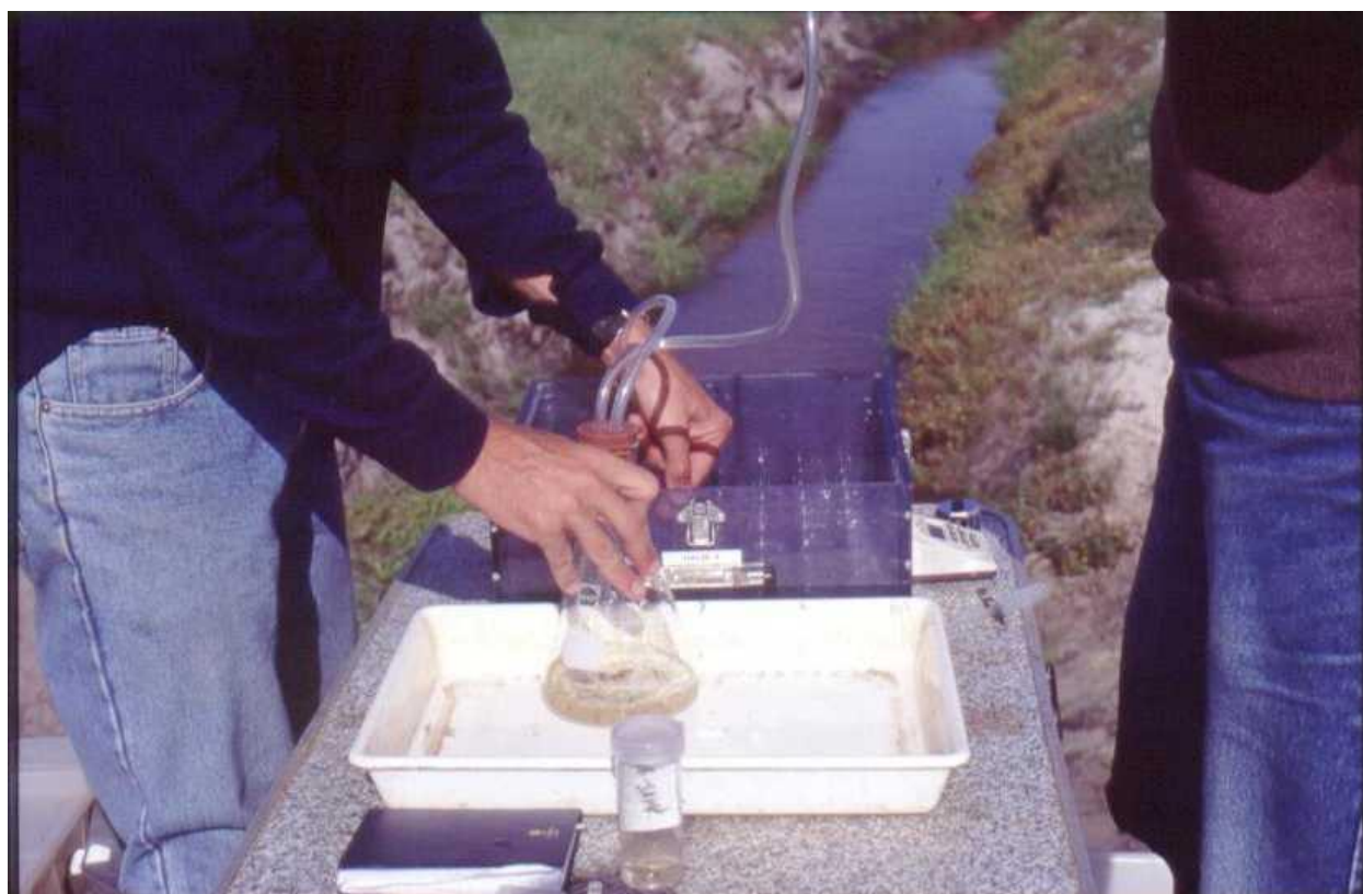
Figure 1. Box subsampler. Sample is being sucked out of a randomly selected cell into conical flask using vacuum created with hand pump (out of sight)
