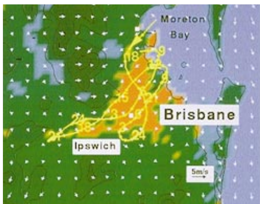
CSIRO computer model simulations of local winds at 100m (white arrows) and associated air trajectories (yellow lines), with time of day marked.
