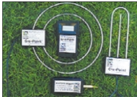
FIGURE 6.21 Gro-Point soil moisture sensor: standard and extended models and handheld reader.
