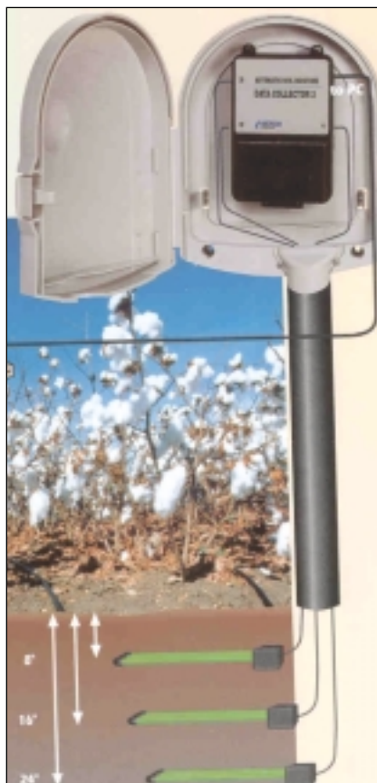
FIGURE 6.15 Netafim soil moisture data collector.
