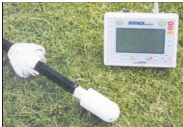
FIGURE 6.9 Sentek Diviner 2000 sensor and display unit.
