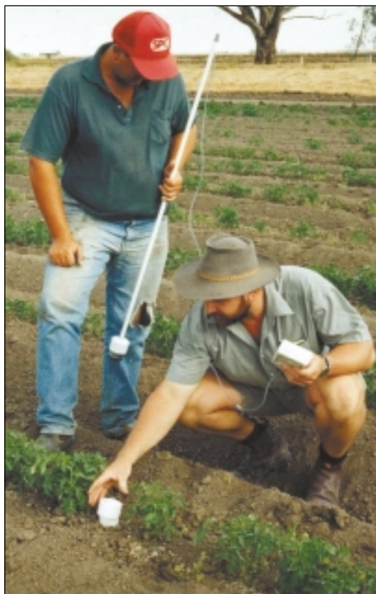
FIGURE 6.11 The Gopher manually operated soil-moisture monitor.
