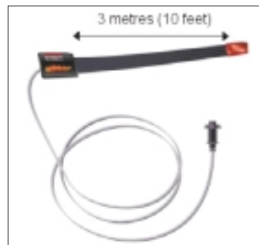
FIGURE 6.20 Aquaflex sensor with high quality data cable and connector.
