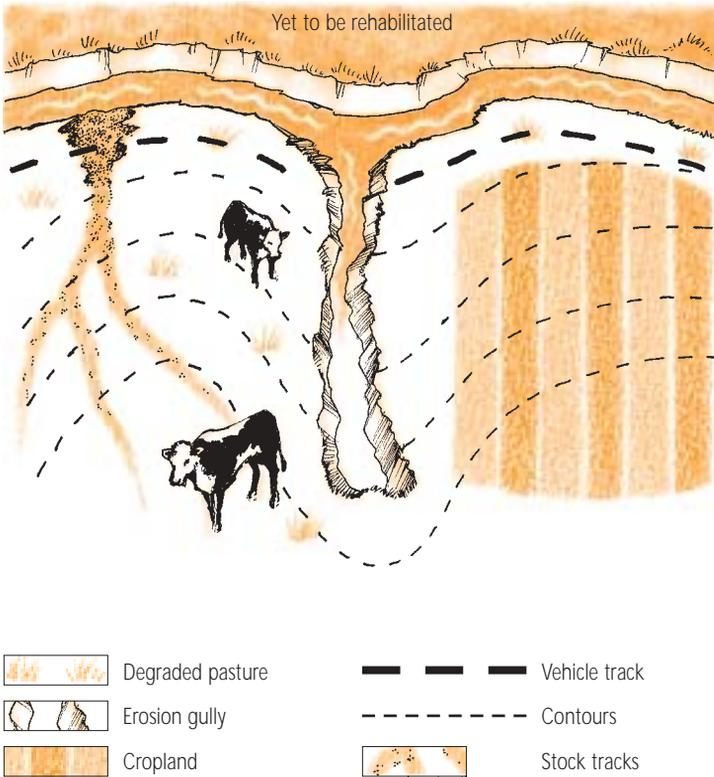
A degraded catchment and riparian land. Significant sediment and nutrient is derived from degraded pasture, poor crop management, unlimited stock access and gully erosion.
