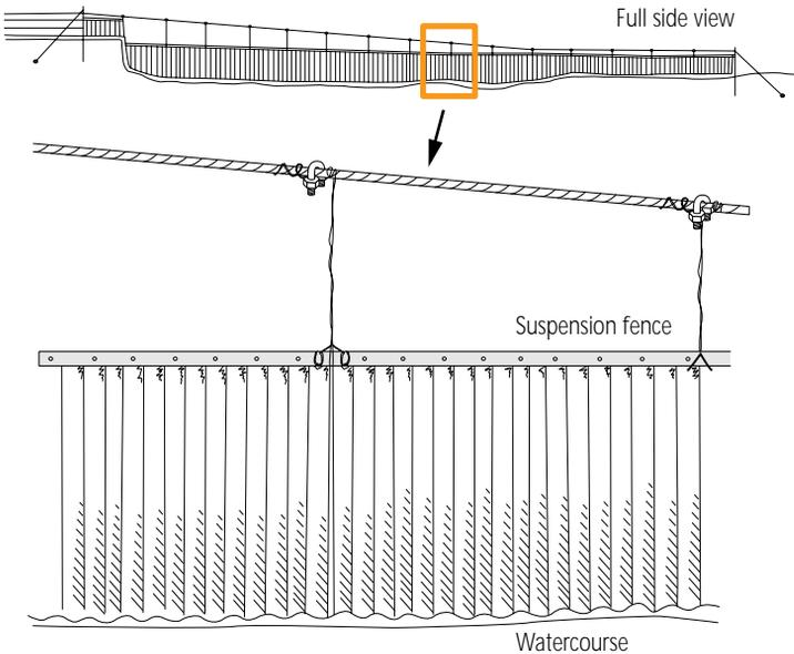
Used galvanised sheets or chain wire mesh suspended from strained cable.
