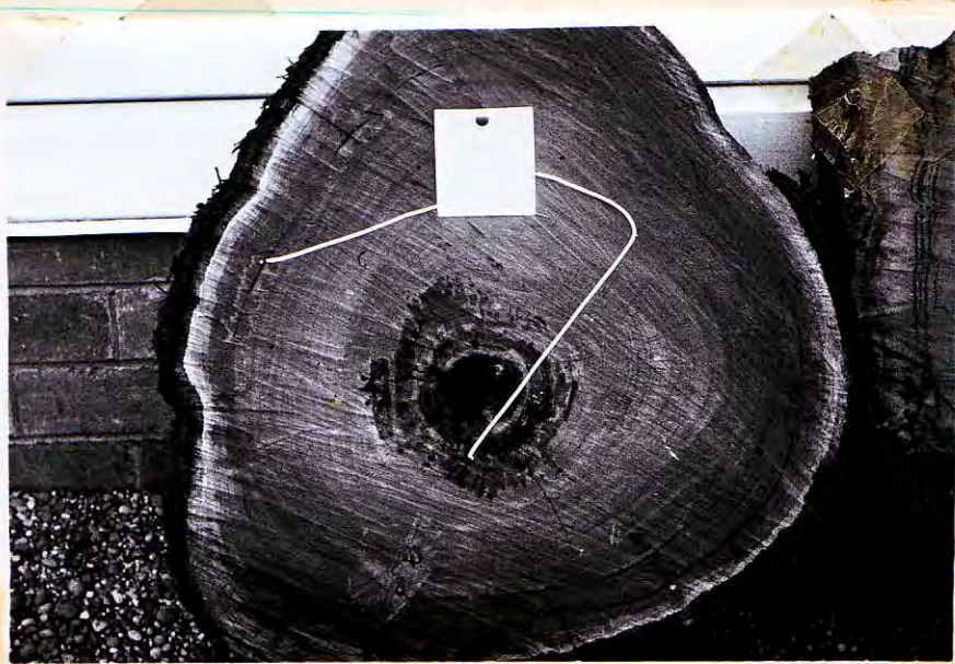
9. Jarrah section showing a) defect due to suppression b) defect due to fire damage most likely.
