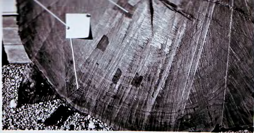
7. Karri section showing a) defects on compression wood side b) rot at an age.
