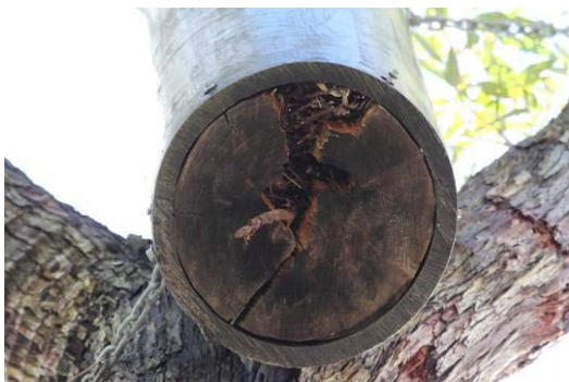
Figure 13: Rotted wooden base of artificial hollow.
