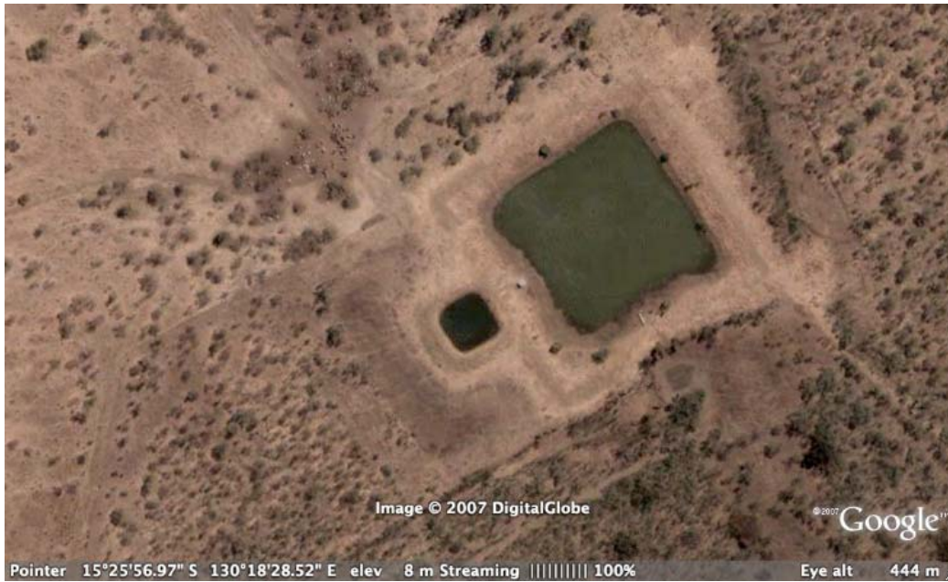
Leichardt tank showing turkey nest dam and larger reservoir tank to the east.
