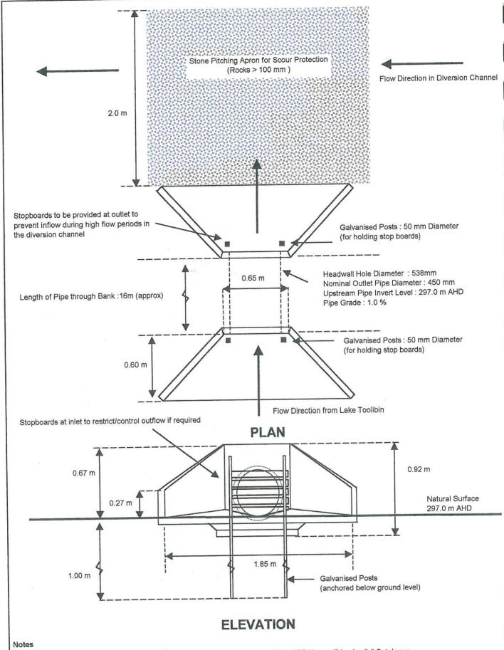
Headwall Dimensions are for a standard precast 450mm diameter pipe headwall via CSR Humes "Headwalls" Catalogue
