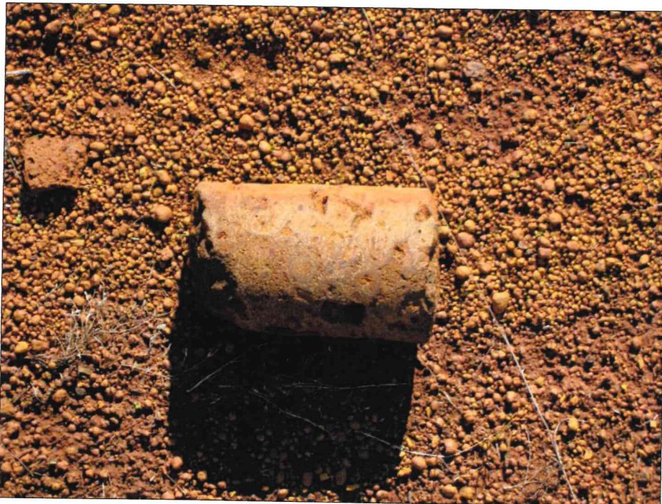
Plate C2: Ruabon Road, Swan Coastal Plain, discarded core sample in road reserve from mineral sand exploration drilling, shows concentric rings as iron-oxides have cemented the original soil. 25/5/2006.
