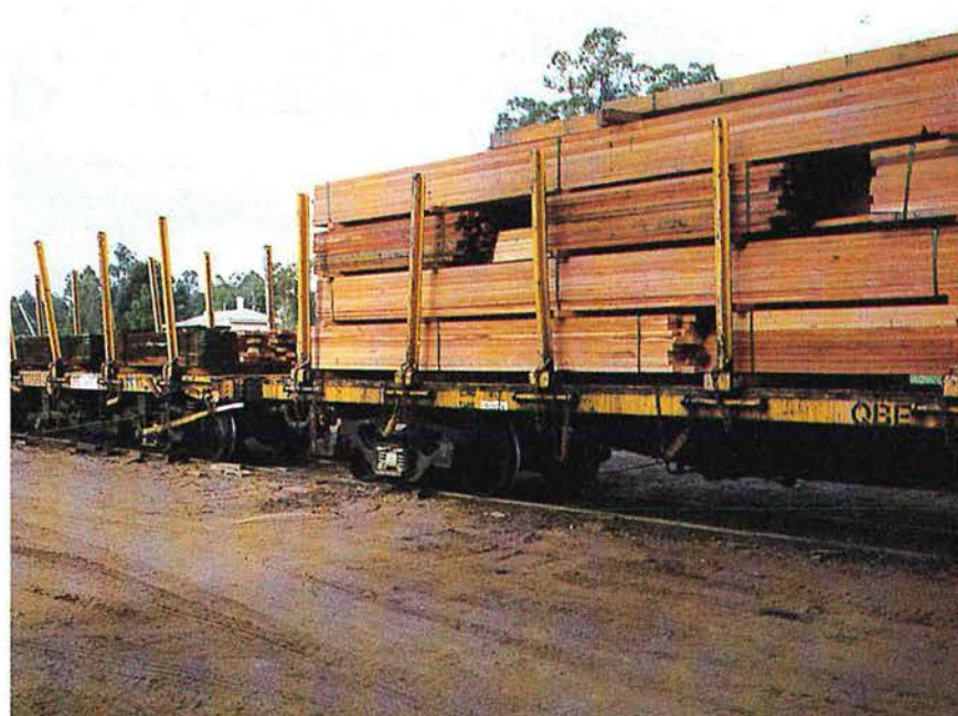
9. Meanwhile the timber from the sorting bench has been strapped into bundles and loaded aboard rail wagons or road trucks to be taken to the customer.
