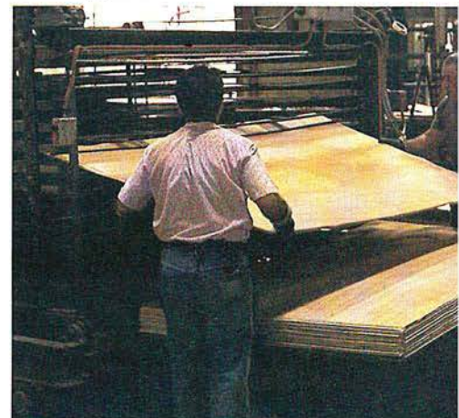
● Workers "lay-up" the sheets of veneer to make plywood.
